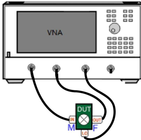
Figure 2. Mixer measurements with a four port VNA
