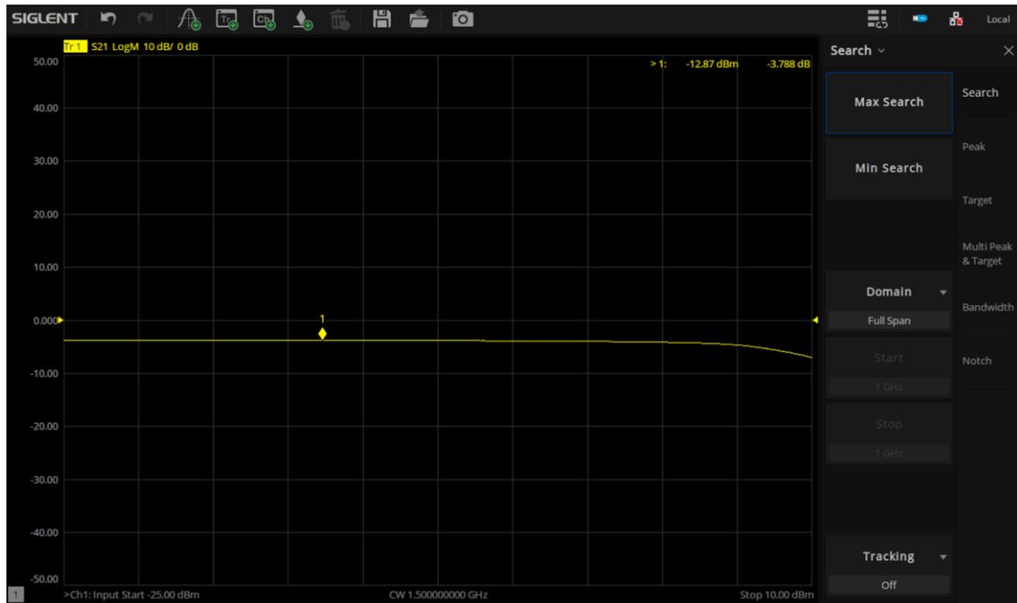
Click **Target** -> **Target Value**, input -4.788, click **Target Search**. The marker reading means at the frequency of 1.5 GHz, when RF input power is 6.821 dBm, the conversion loss/gain of the mixer is -4.792 dB. It starts to get into compression area.
