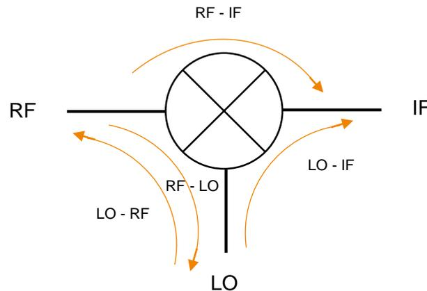
Figure 5. Signals leakage or feed-through
