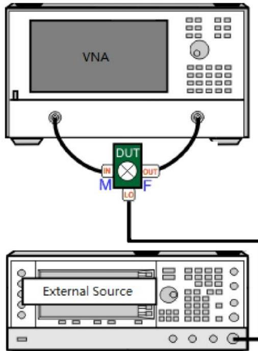
Figure 3. Mixer measurements with a two port VNA
