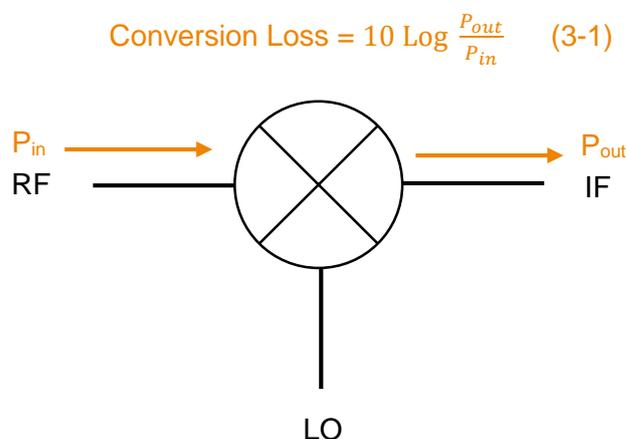
Figure 4. Mixer Conversion Loss/Gain
