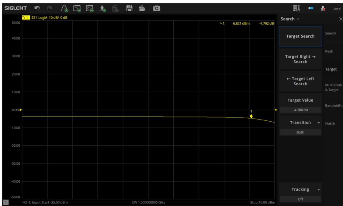
c) Conversion Loss / Gain as a function of LO power level.
