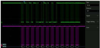
Display the decoded characters through the events list. Bus protocol information can be quickly and intuitively displayed in tabular form. I<sup>2</sup>C, SPI, UART, CAN, LIN, CAN FD, FlexRay, I<sup>2</sup>S, MIL-STD-1553B, SENT and Manchester are supported
