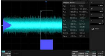
The Waveform Histogram feature provides a statistics view of the waveform in horizontal and vertical directions
