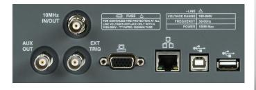
USB 2.0 Host, USB 2.0 Device (USBTMC), LAN 10M/100M (VXI-11, telnet, socket, web), Pass/ Fail, Trigger Out, 10 MHz In/Out and VGA output
