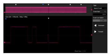
The SDS5000X can search events specified by the user in a frame. Events flagged by the Search can be recalled automatically using Navigate. It can also navigate by time (delay position) and history frames
