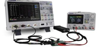
The SDS5000X can control the USB AWG module or a standalone SIGLENT SDG generator, to scan the amplitude and phase frequency response of the DUT, and display the data as a Bode Plot. This makes it possible to replace expensive network analyzer in some applications The Power Analysis option provides a full suite of power measurements and analysis, which greatly improve the measurement efficiency in switching power supplies and power devices design
