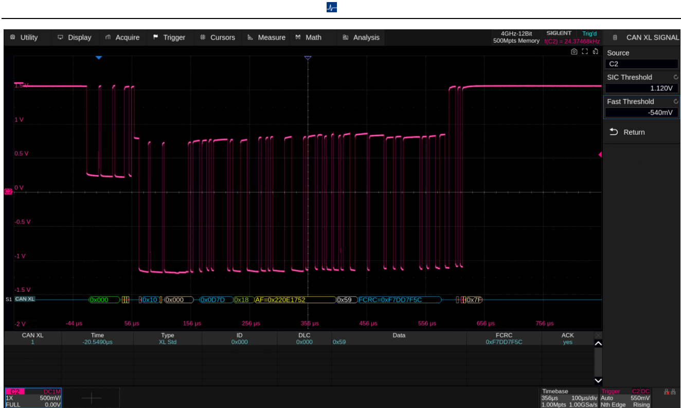
Figure 7 CAN XL Fast Mode Protocol signal Settings
