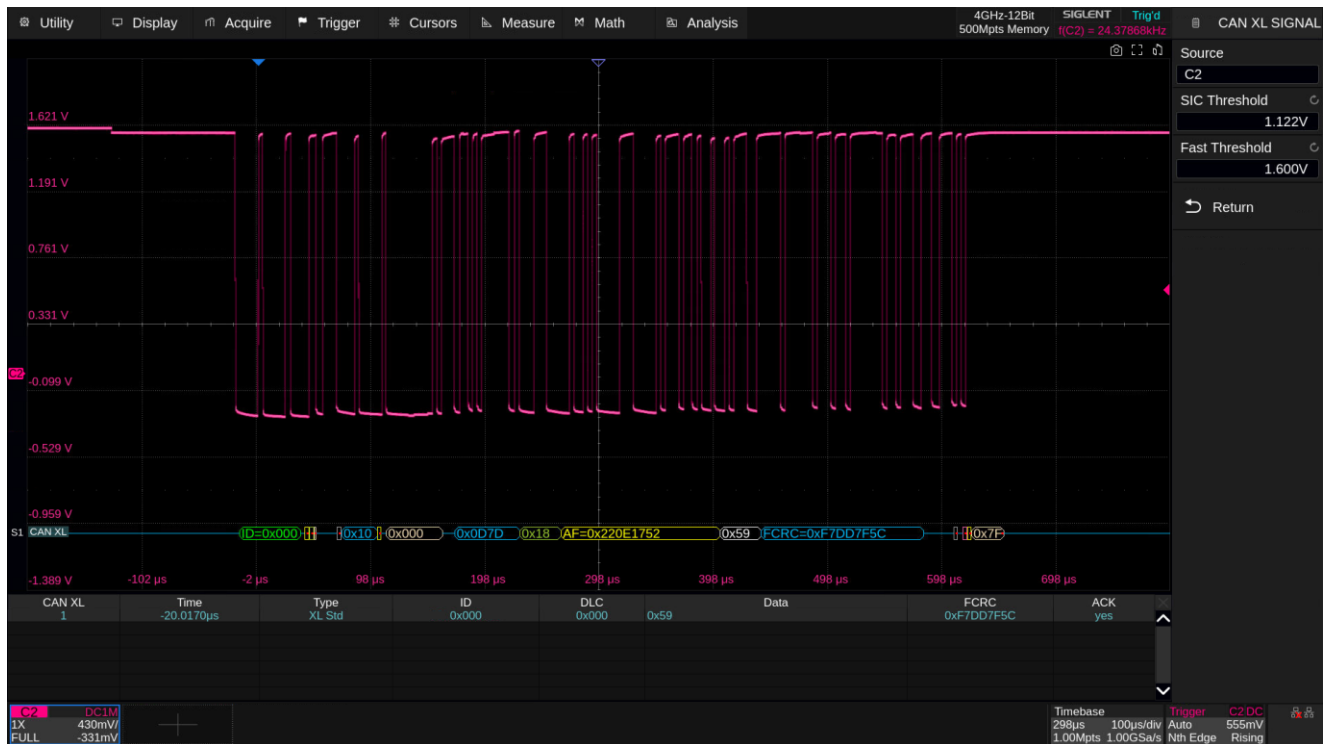
Figure 9 CAN XL SIC Mode Protocol Signal Setting
