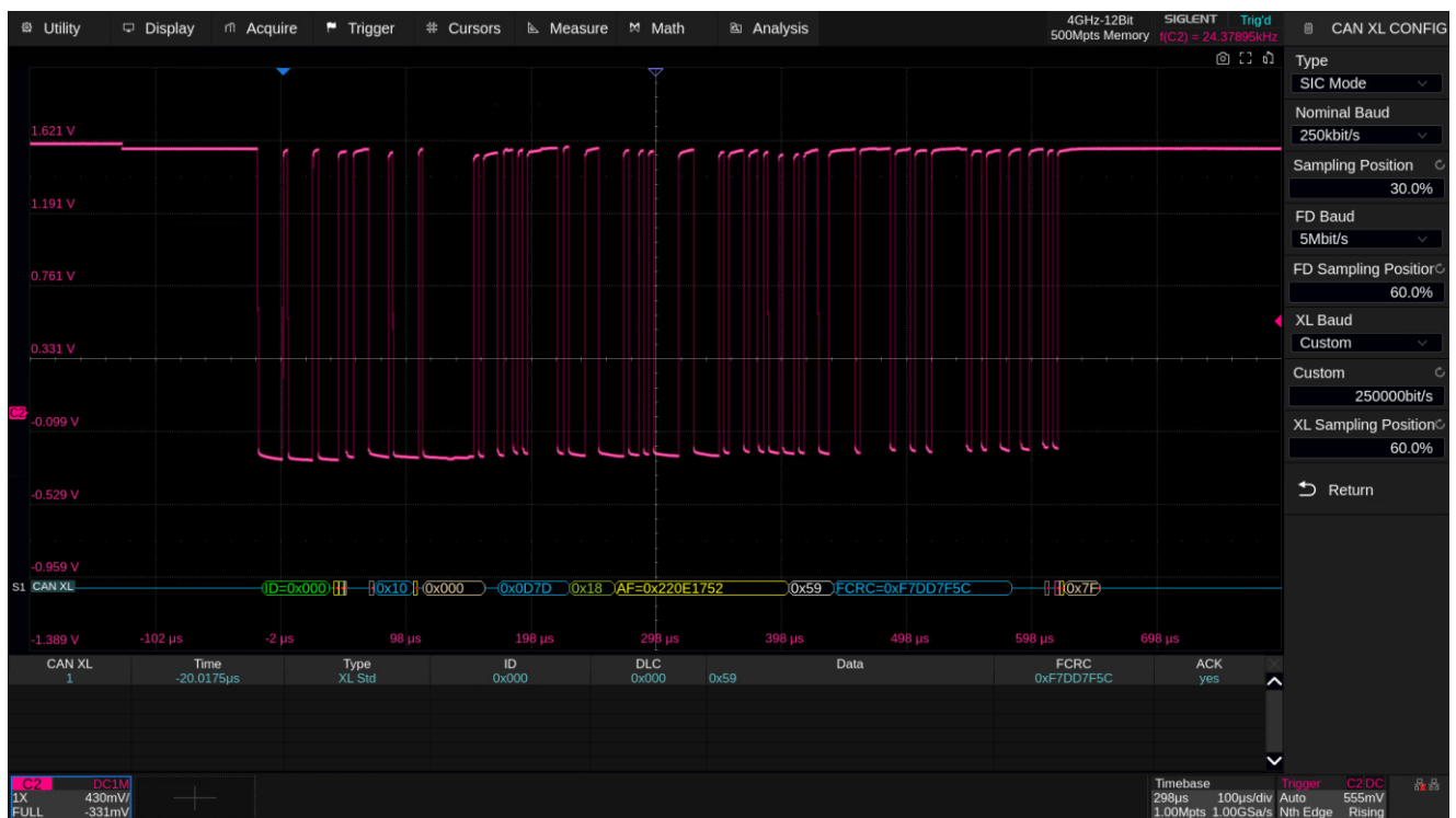
Figure 10 CAN XL SIC Mode Protocol Configuration Settings
