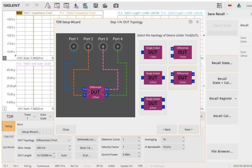
**Figure 2: DUT Topology in the TDR Setup Wizard**
