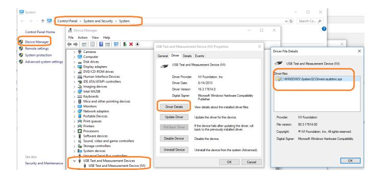
As you can see, a correctly configured and working USB Test and Measurement device will use the AUSBTMC.SYS driver.
