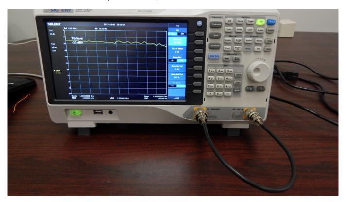
The average output should be equivalent to the setpoint and the flatness should be within 3dB of that setpoint. If not, there is likely an issue with the TG, RF input, Cable, or connectors.
