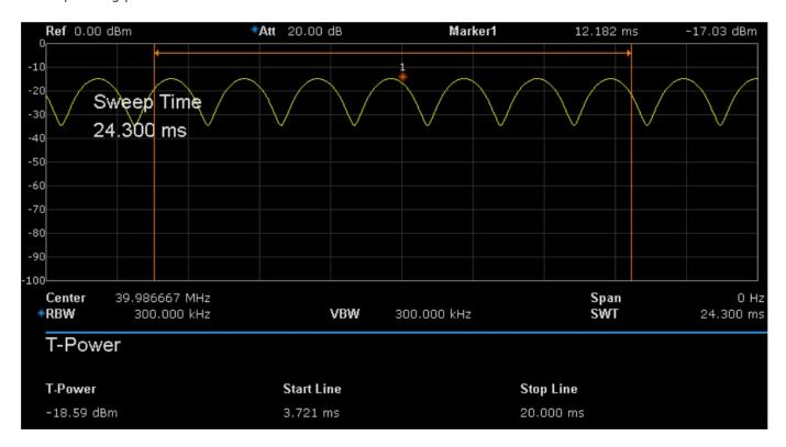
**T-Power:** The power of the signal from the start line to the stop line.
