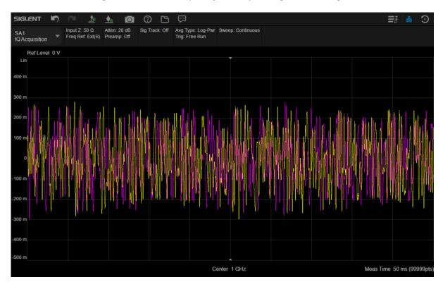
(3) Click <u>AMPTD</u>, Adjust the reference level, the scale and measurement time to better display the I/Q waveform on the screen.
