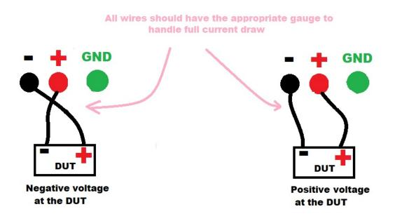
**Grounded Wiring Configuration:**
