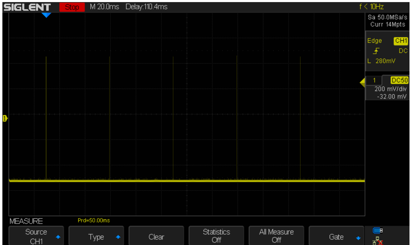
Figure 4 Five successive pulse signals acquired by traditional methods
