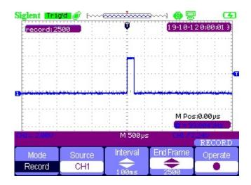
You can press OPERATE at any time to stop recording.
