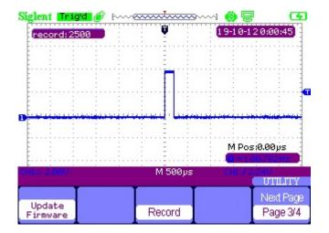
3. From the record menu, change the MODE to RECORD, select the source, and set the number of frames you wish to record. Here, we have it set to record 2500 frames, which is the maximum. To begin recording, simply press the OPERATE button.
