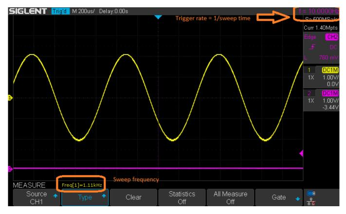
The frequency marker will output a pulse at the same time that the sweep frequency meets the setpoint for marker frequency.
