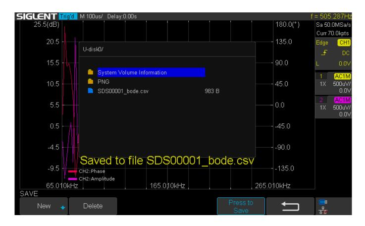
5. When you want to recall, insert the USB memory device or recall from the internal memory. Open the Bode II application on the scope, click on Data, press Recall, and select the file of interest :
