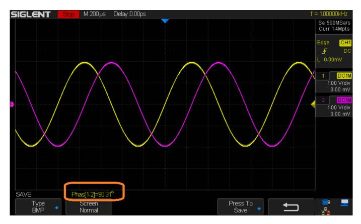
Step 2: Send "C1-C2:MEAD? PHA" to activate phase measurements between CH1 and CH2.
