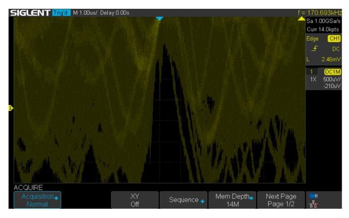
The noise on the 500 uV/div vertical scale is dominating the screen.. so we can adjust the scale until we get some headroom... 5 mV/div is better..
