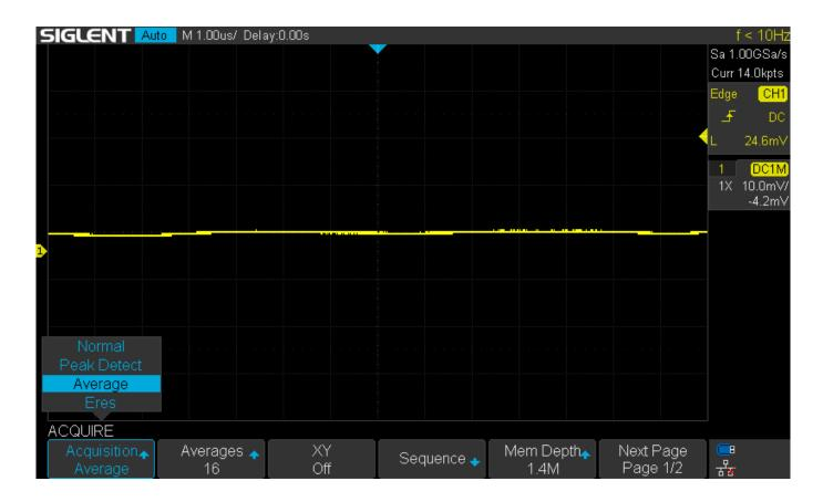
4. We can also use the Zero function of the probe to minimize the DC offset of the measurement. Now, our open-circuit voltage average is near 0 V.
