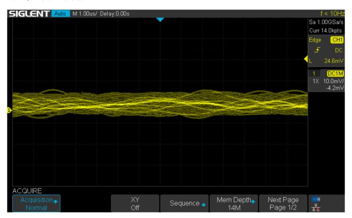
3. Now, let's enable averaging. For continuous (DC) outputs or repeated waveforms, averaging can be used to minimize random noise:
