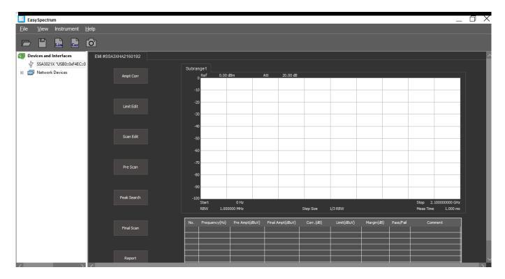
3. Ampt Corr: Amplitude correction can be activated to mathematically adjust the collected data to account for cable/adapter losses as well as antenna gain factors.
