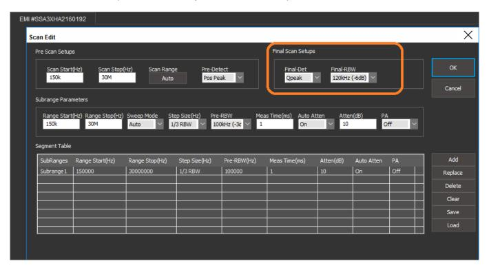
The Final Scan operations are applied to each peak in the peak table only. The SSA is placed into zero span mode centered on the peak frequency from the table and the scan commences.
