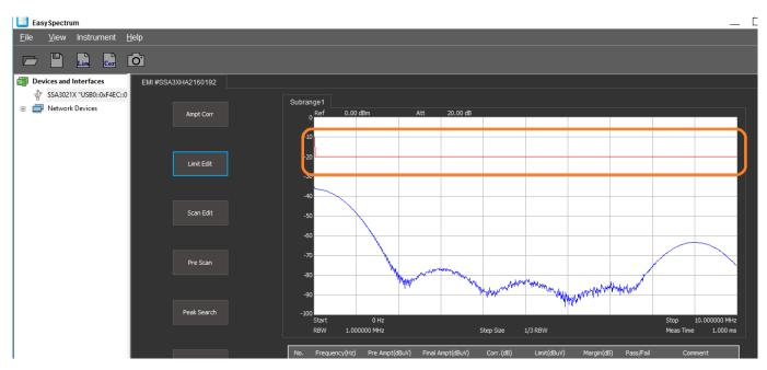
5. Scan Edit: Configure the scan which is broken up into three distinct parts. While they can be configured in many different ways, here are oursuggested settings for preliminary scans:
