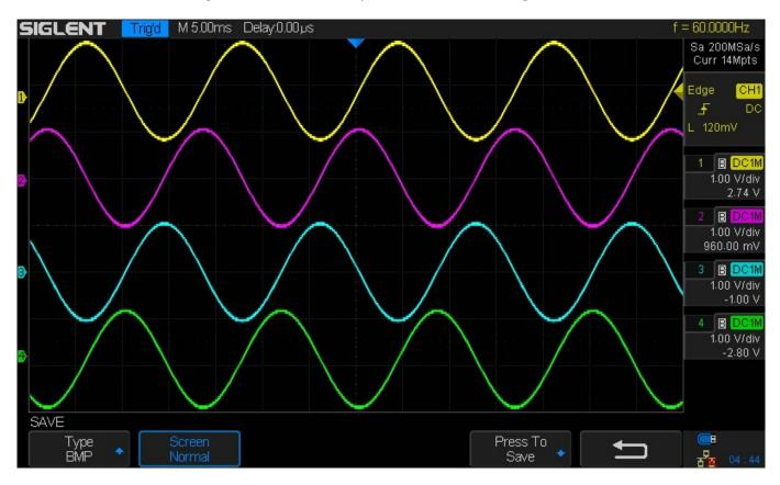
If CH1 and CH2 are out of phase for either unit during set up choose EqPhase from the menu in order to align the two phases.
