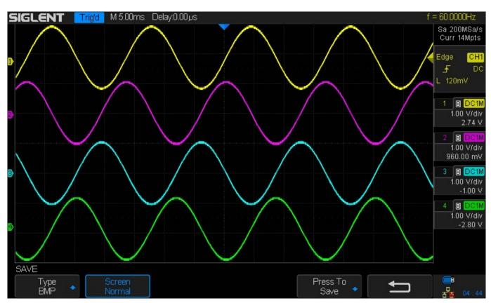
If CH1 and CH2 are out of phase for either unit during set up choose EgPhase from the menu in order to align the two phases.
