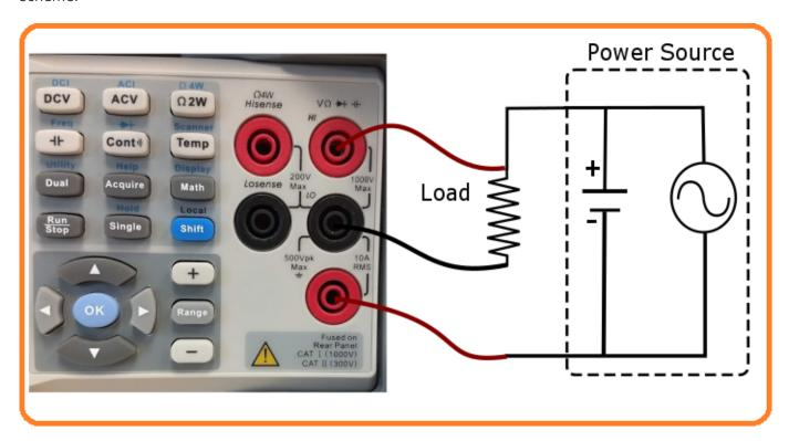
NOTE: The resistance of the test leads and the internal resistance of the ammeter (current measurement) will add error to the measurement using this technique.
