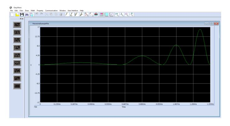
Now, download the file to the instrument. The front panel of the AWG will indicate that the waveform is an ARB and will have a picture representing the new waveform on the front panel:
