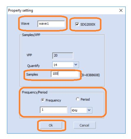
**NOTE:** Set the number of samples based on the resolution and the output sample rate that your application requires. A good starting point is to use 10 data points for the shortest feature you wish to create.
