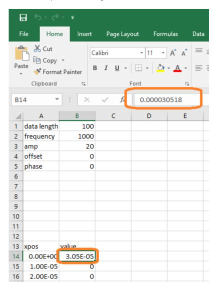
3. The data length value (cell B1) must match the total number of points in the column labeled value that starts at column B, row 14.
