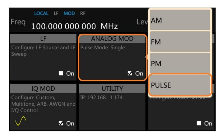
To output a single pulse just set the pulse mode to Single:
