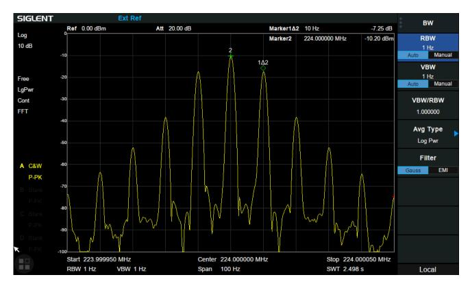
In addition to the previous measurements of channel power (CP), adjacent channel power (ACPR), occupied bandwidth (OBW), TOI and waterfall diagram (monitor), the harmonic and carrier-to-noise ratio (CNR) measurements are now also included in AMK option. The EMI filter bandwidth is now 200 Hz, 9 kHz, 120 kHz and 1 MHz. The SSA3000X Plus shows more powerful measurement capability.
