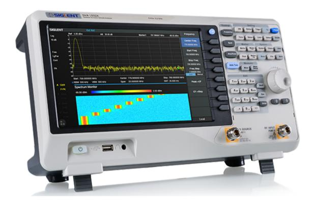
SIGLENT Technologies presents the SVA1032X as a novelty from the product group of spectrum & vector analyzer. Compared to SVA1015X, not only frequency range is extended, but also performance and RF specs. The spectrum analyzer frequency range is 9 kHz – 3.2GHz, vector network analyzer frequency range is 100 kHz – 3.2 GHz. Furthermore, the optional vector network analysis (VNA) function will be included in the SVA1015X model as also standard.
