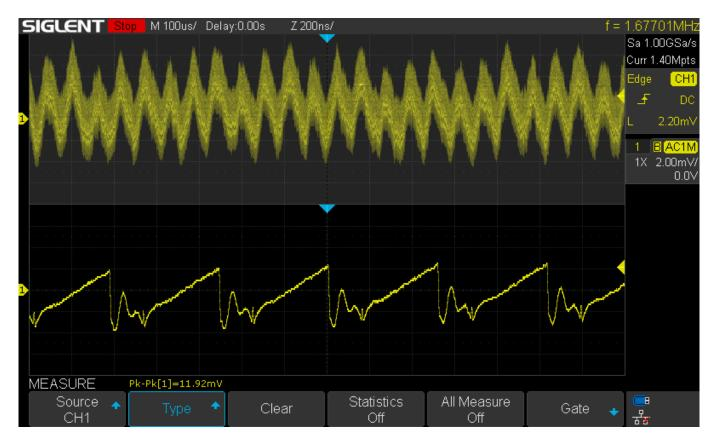
Want to test a power supply? Using the AC coupling measurement function, you can clearly see the AC component of the signal. With the SDS1104X-U, SIGLENT delivers another cost-effective electronic test and measurement solution.
