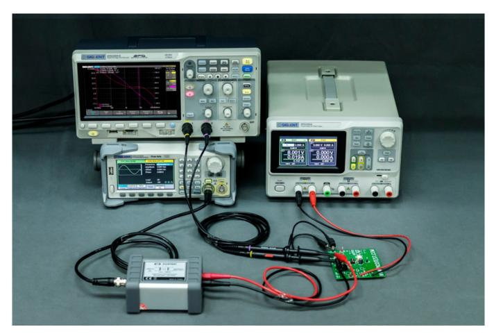
Here is a new powerful but low-cost solution for you. The SIGLENT SDS2000X-E series oscilloscope with its newly released Bode Plot II feature together with a SIGLENT SDG2000X series function generator offers a very flexible and easy-to-use power supply control loop measurement system. Click the following link for an application note about the basic principles for making the stability measurement and how to use these instruments to make the measurement.
