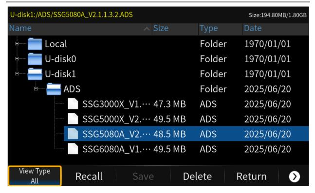
4. The system will first decompress and verify the upgrade package. If the upgrade package passes the verification, the instrument will automatically upgrade.
