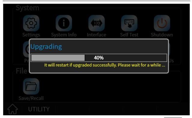
5. After the instrument reboots, check the version number through the Utility -> System Info to confirm if the upgrade is successful.
