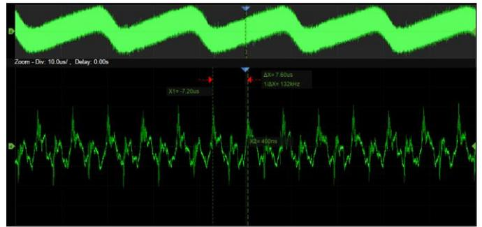
Utilizing a hardware-based Zoom technique and record length up to 200 Mpts, users can select a slower timebase without compromising the sample rate and then quickly zoom in to focus on the area of interest.
