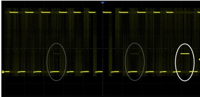
With a waveform update rate of up to 120,000 wfms/s, the oscilloscope can easily capture low-probability events. In Sequence mode the waveform capture rate can reach 500,000 wfms/s.
