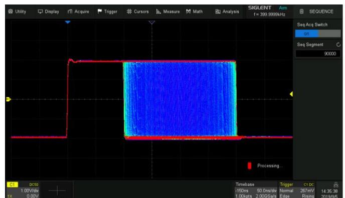
Segmented memory collection will store the waveform into multiple memory segments (up to 90,000) and each segment will store a triggered waveform together with the dead time information. The interval between segments can be as small as 2 μs. All segments can be played back at an arbitrary frame rate using the History function.
