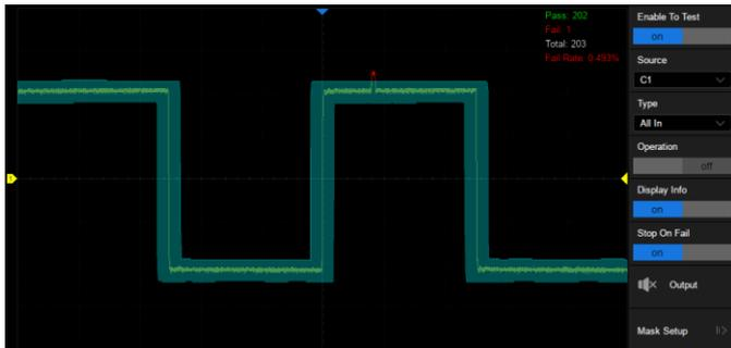
The SDS2000X Plus utilizes a hardware-based Mask Test function, performing up to 80,000 Pass / Fail decisions each second. It is easy to generate user defined test templates which the signal trace can be continuously compared to. The failed frames can be automatically stored as history frames or screen shots, making it suitable for long-term signal monitoring or automated production line testing.
