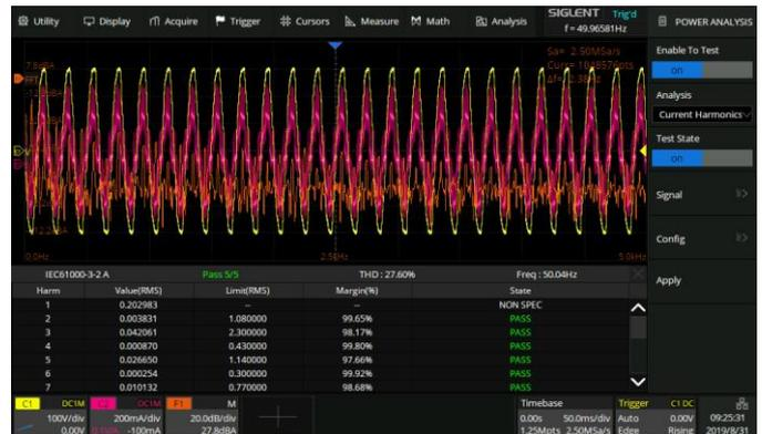
The Power Analysis option provides a full suite of power measurements and analysis, thus improving the efficiency of measurement in switching power supplies and power device designs.
