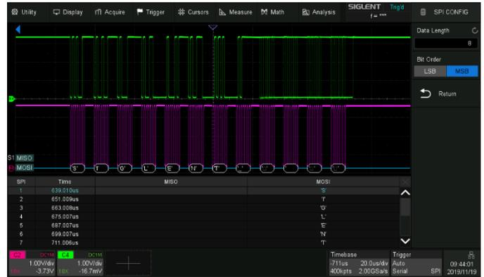
In addition to the decoder lanes correlated to the waveform, bus protocol information can be displayed in tabular form. I<sup>2</sup>C, SPI, UART, CAN, LIN, CAN FD, FlexRay, I<sup>2</sup>S, MIL-STD-1553B, SENT and Manchester are supported.
