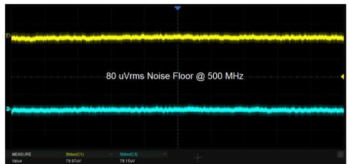
500 MHz bandwidth (at 2 GSa/s sample rate with 500 MHz bandwidth option).
