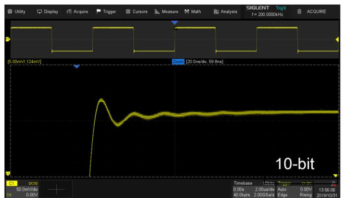
10-bit mode combined with Zoom shows you more details and less noise on the waveform.
