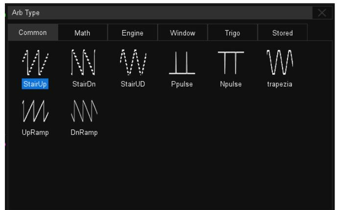
The built-in DDS waveform generator can output waveforms with up to 50 MHz frequency and  $\pm 3$  V amplitude. Six basic waveforms together with multiple types of predefined waveforms and as user defined arbitrary waveforms are supported.
