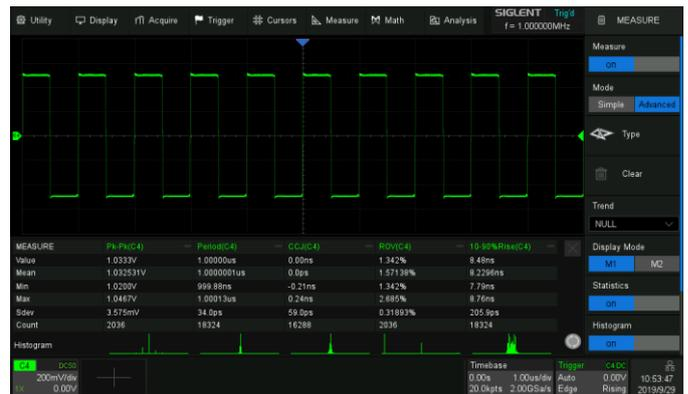
Measurements can be performed within a specified gate period. Measurements on Math, Reference and History frames are supported.
