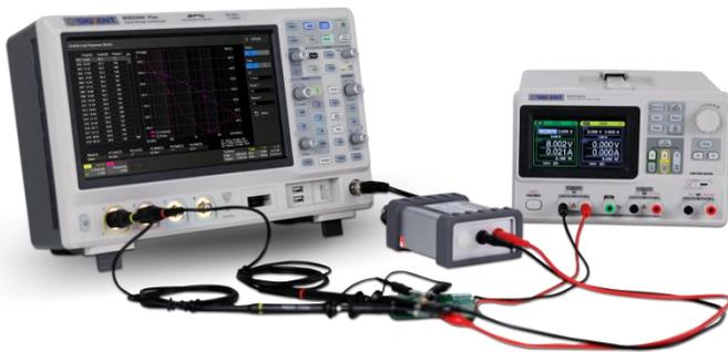
The SDS2000X Plus can control the built-in waveform generator or any stand-alone SIGLENT SDG device to scan the amplitude and phase response over frequency of passive or active circuits. The data is presented as Bode Plot. This makes it possible to replace expensive network analyzers in less demanding applications.
