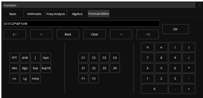
Two Math traces, support FFT, +, -, x, ÷, d/dt, ∫dt, √, Identity, Negation, |x|, Sign, e<sup>x</sup>, 10<sup>x</sup>, ln, lg, Interpolation, average, ERES, and formula editor.
