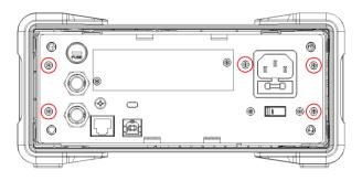
7. Remove the cable plug connected to the front panel.
