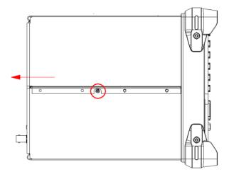
Remove the cable plug (in the red circle and yellow box shown below) connected to the main body.
