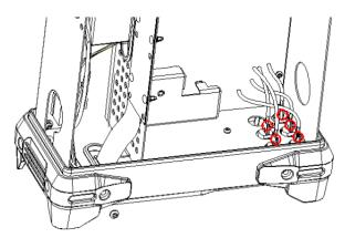
8. Remove the cable and unscrew all the screws then you can remove the PCBA.
