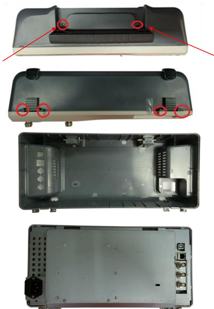
Figure 4-1 Removing the Rear Panel Screws
