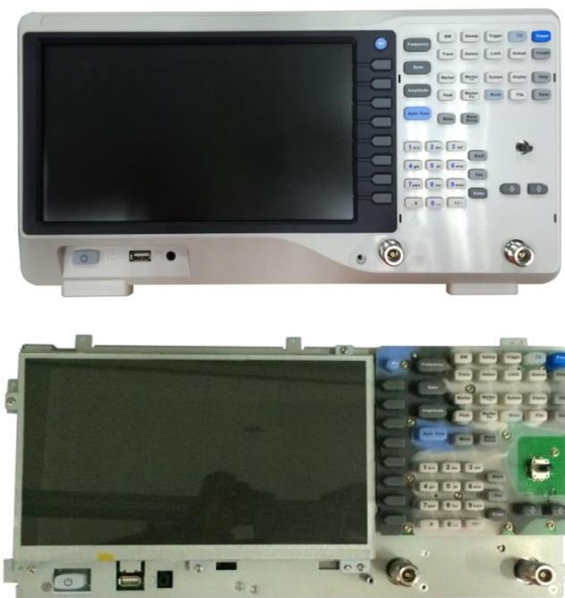
Figure 4-2 Removing the front panel
