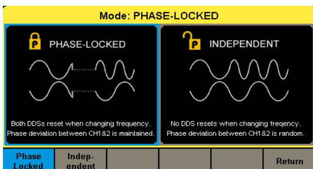
"Phase-Locked" mode automatically aligns the phases of each output. While "Independent" mode permits the two channels to be used as two independent generators. Independent mode also smoothes parameter (frequency, amplitude) changes made to an active channel.
