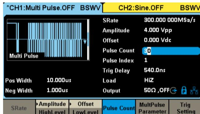
Built-in dual pulse output function, combined with siglent's oscilloscope, can quickly measure the switching parameters and dynamic characteristics of power devices without the need for host computer software.
