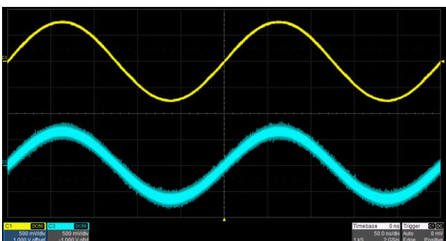
Wideband Gaussian noise can be easily added to other waveforms to simulate real-world scenarios in which the signal contains a large degree of noise.
