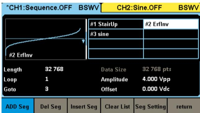
Easily set the number of cycle times for each waveform and the order of waveform playback.
