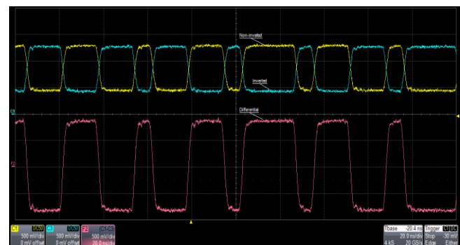
Preset common logic levels such as TTL, LVCMOS, LVPECL and LVDS. An added differential mode provides an easy way to generate differential signals using the both channels.
