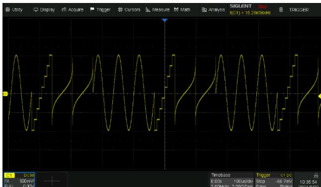
Provides sequence playback function to easily meet various testing needs. Maximum waveform storage depth reaches 20 Mpts/ch.
