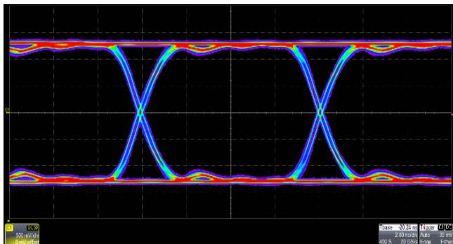
PRBS3 ~ PRBS32 with finely adjustable 10<sup>-6</sup> bps ~ 300 Mbps bit rate and 1 ns ~ 1us edge.
