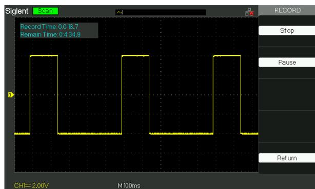
The digital recorder is able to record data in real-time and without any dead time. SDS1000DL+/CML+ supply 7 M of memory for the recorder and support a USB disk.
