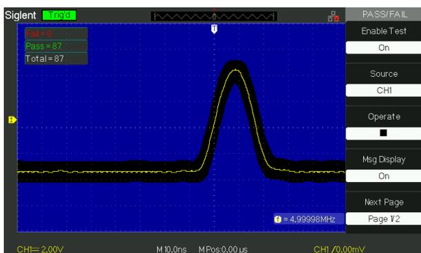
With easy to generate user-defined test templates, the SDS1000DL+/CML+ compares the current measured trace to the template mask trace making it suitable for long-term signal monitoring or automated production line testing.
