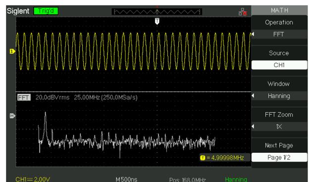
SDS1000DL+/CML+ provides 5 kinds of math operation: +, -, \*, /, FFT, supporting channel waveform and FFT waveform in either split display windows or both signals appearing on the full screen.
