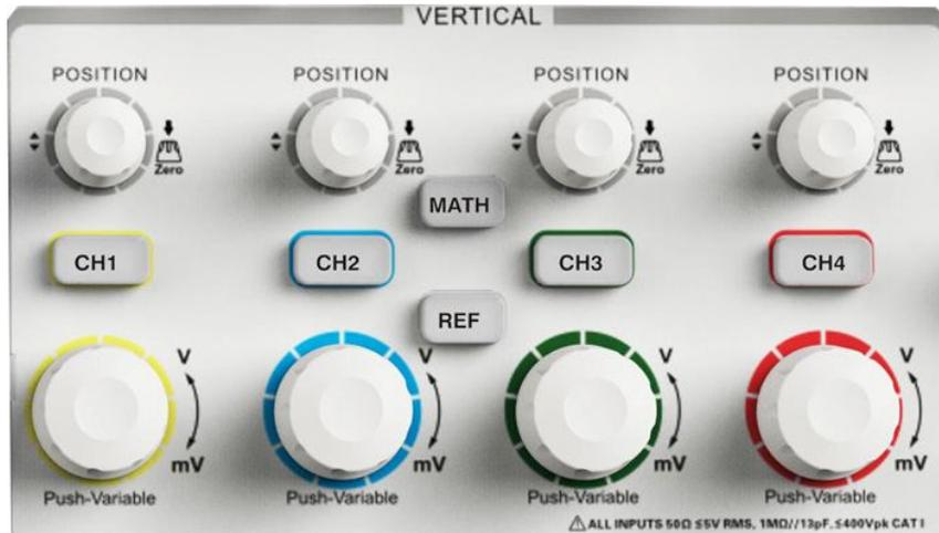
**CH1** **CH2** **CH3** **CH4** : Input channels. These four channels are marked with different colors to distinguish different input channels and their waveforms. Press the channel button will turn on the corresponding channel as well as its menu, and press it twice continuously will turn off the channel.
