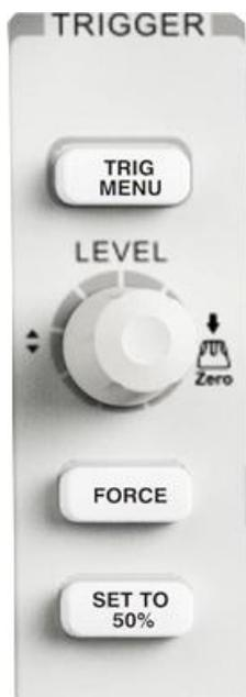
**TRIG MENU** : Press the button to open trigger menu under which five trigger modes are supported.
