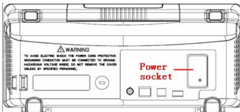
Note: In want of replacing the fuse, please return the instrument to the factory that produced it to have it repaired by qualified service personnel authorized by **SIGLENT**.
