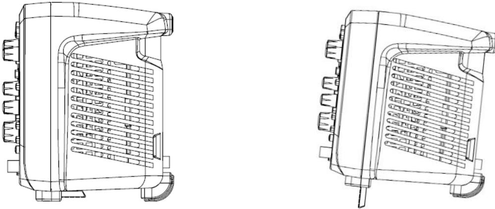
**Figure 3** Adjust the Supporting Legs
