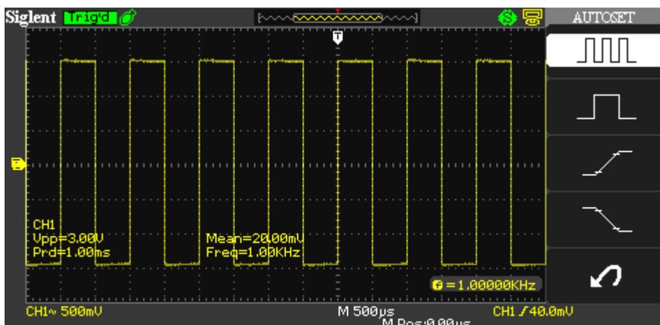
6. Test the other channels in the same method. If the actual square waveforms does not match that in the figure above, please perform "Probe Compensation".
