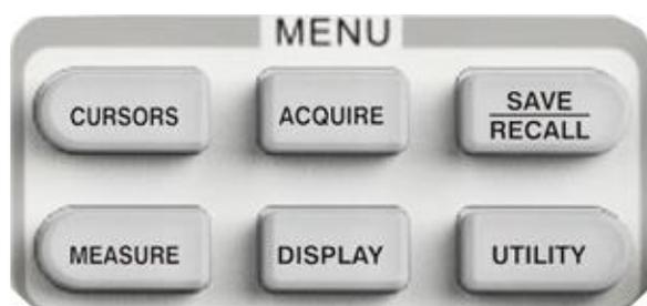
**CURSORS** : Press the button to enter the cursor measurement function menu. The instrument provides three measure modes: Manual measurement, Track measurement and Auto measurement.
