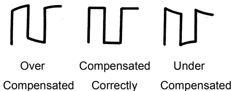
3. Use a nonmetallic driver to adjust the low-frequency compensation adjustment hole on the probe until the waveform changes to be correct as the figure above.
