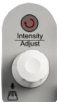
**Adjust waveform brightness:** While the light above the knob is dark, revolving the knob will adjust the brightness of the waveform, which ranges from 30% to 100%. Turning clockwise means increase while counterclockwise means decrease. You can also select “intensity” in “DISPLAY” menu and then revolve the knob to adjust the brightness of the waveform.
