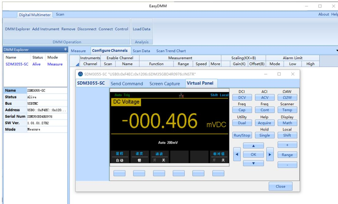
Diagram 3-19 The Main Interface of EasySDM
