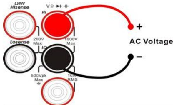
Diagram 2-9 Sketch Map for Measuring AC Voltage
