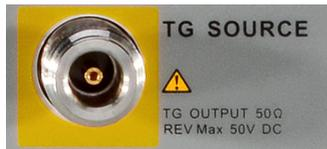
To avoid damage to the tracking generator, The reverse DC voltage must not exceed 50V
