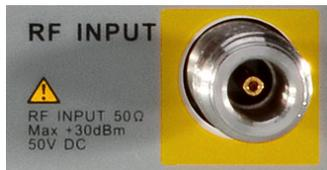
To avoid damage to the instrument, make certain that the input signal to the RF input port does not contain more than 50 Volts DC. The AC (radio frequency) input signal component should not exceed a maximum continuous power level of +30dBm.
