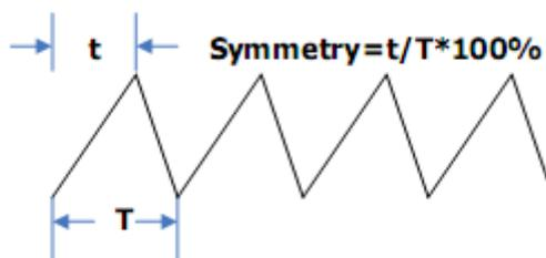
1. Press **Waveforms** → **Ramp** → **Symmetry** , to set the symmetry.
