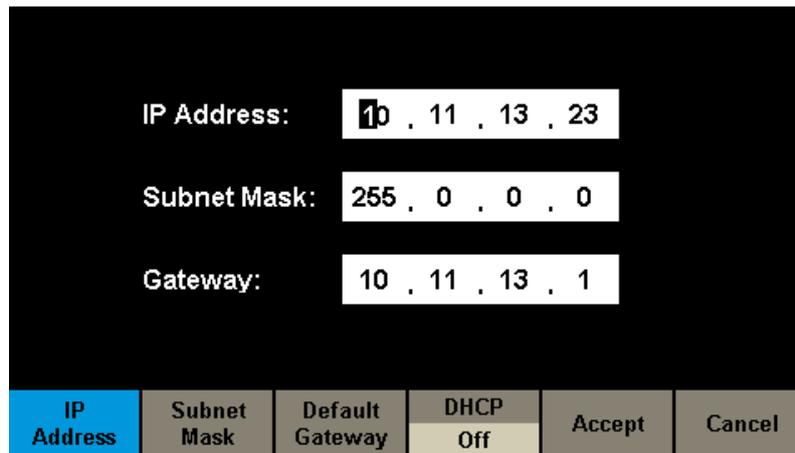
The image shows a LAN Settings Interface with a black background. It features three input fields for network configuration: IP Address (10 . 11 . 13 . 23), Subnet Mask (255 . 0 . 0 . 0), and Gateway (10 . 11 . 13 . 1). Below these fields is a navigation bar with six buttons: IP Address (highlighted in blue), Subnet Mask, Default Gateway, DHCP Off (highlighted in yellow), Accept, and Cancel.
