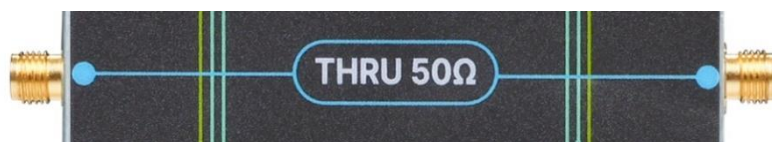
Figure 3-1 Schematic diagram of 50 Ω short through line
