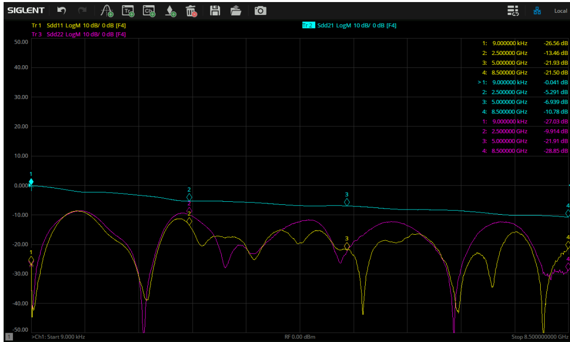
Figure 4-18 Test result of differential impedance transformation line
