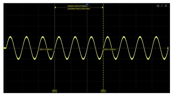
Fixed delay, timebase is changed to 100 ns/div, the value of MX1 and Mx2 cursors (-200 ns, 100 ns) remains fixed. The grid number of MX1 and Mx2 cursors is changed to -2div, 1div.
