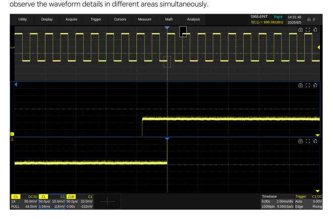
The area not covered by the gray background in the main waveform area is the range to be zoomed in (zoom area). Click the descriptor box of the zoom trace to recall the quick dialogs for setting the vertical and horizontal parameters of the zoom window.
