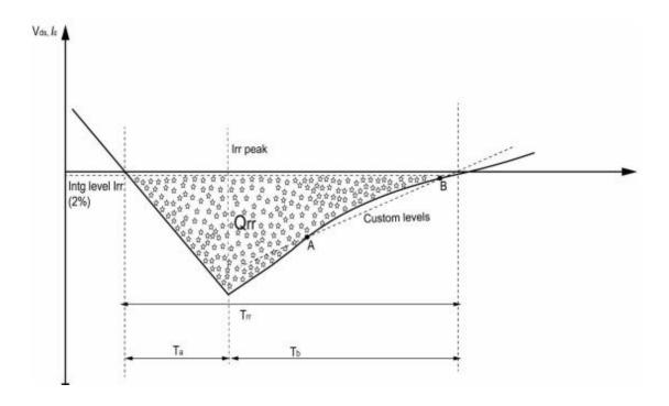
Trr -- Measures the reverse recovery time using configured levels.
