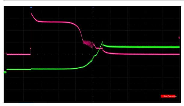
Voltage and current waveforms on the MOSFET at power-up
