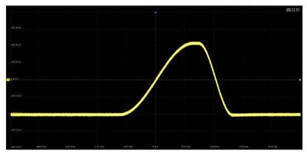
In the example, 43231 pulses can be obtained with the sample rate of 5 GSa/s at the maximum memory depth.
