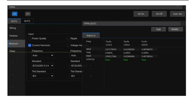
In the chart dialog box, check the table or bar chart to view the details of each phase harmonic, including harmonic effective value, standard, tolerance, and judgment results. In the bar chart, harmonic results are highlighted in green under passing conditions and in red when exceeding test limits.
