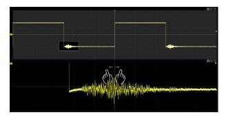
Adjust the horizontal scale of Zoom window by horizontal pinch and spread in the zoom area of the main window or the Zoom window.
