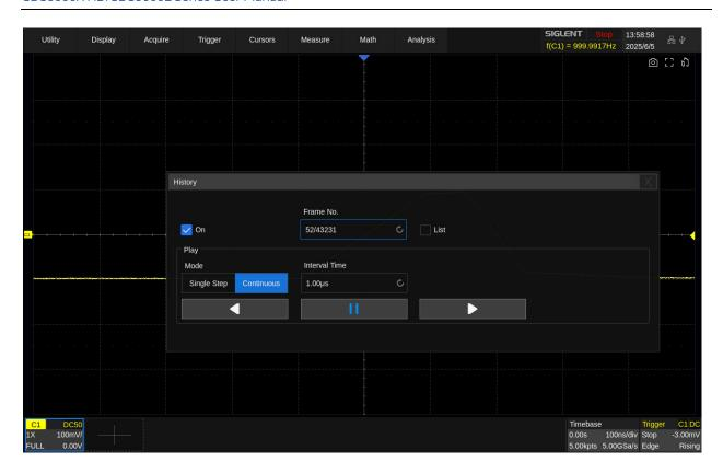
Click the List area and turn on the list. The time label corresponding to the 52th waveform is displayed. The time resolution is microseconds. Time label types include AcqTime or  $Delta\ T$ , AcqTime corresponds to the absolute time of the frame, synchronized with the real-time clock of the oscilloscope; Delta T is the acquisition time interval between adjacent two frames, it is shown as 40ms in the following diagram, which is consistent with the period of the actual waveform.
