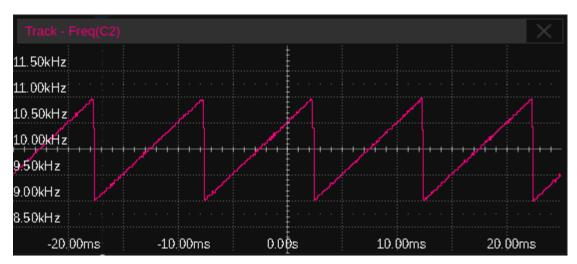
The upper limit of the statistic number in a frame is set in Measure > Statistics > Config > AIM Limit , which means the values exceeding the limit will not be shown in the track plot. The upper limit is 1,000 by default and can be set to up to 100,000.
