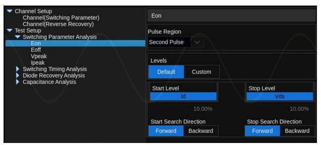
**Eoff** — Measures the energy dissipated by the power device during turn-off. By default, measured on the first pulse width as defined by the standard.
