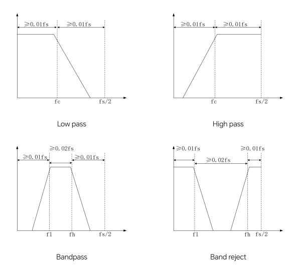
Take a Low pass filter as an example. It requires that the corner frequency (fc) is not less than 0.01\*fs (i.e. fc  $\geq$  0.01\*fs), and the 0.01\*fs wide roll-off does not exceed the 1st Nyquist zone (i.e. (fs/2) - fc  $\geq$  0.01fs). If fs = 5 GSa/s, then the legal range of the corner frequency (fc) is 50 MHz~2.45 GHz
