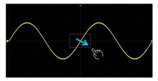
Draw a rectangular box to create a zone or a histogram region. At the beginning of the gesture keep the angle close to 45° so it can be recognized as the drawing box gesture
