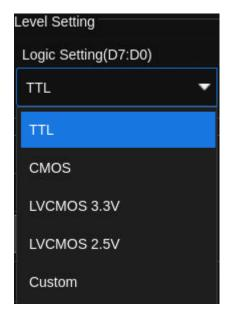
The configurable logical level includes TTL, CMOS, LVCMOS 3.3 V, LVCMOS 2.5 V, and Custom.
