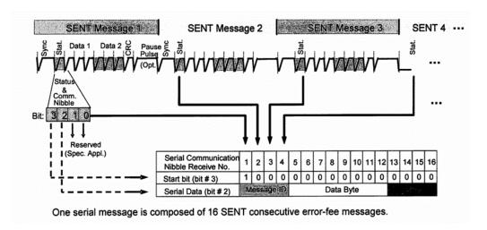
The serial message frame contains 21 bits of payload data. Two different configurations can be chosen
