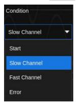
**Start** -- The oscilloscope will be triggered at the start of the message (after 56 Sync ticks). You can select the type of message: Fast Channel Message, Slow Channel Message, or any.
