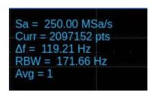
FFT sample rate (Sa): FFT operation results present the first Nyquist zone (DC ~ Sa/2) of the frequency spectrum. Be aware that the FFT sample rate may be inconsistent with the sample rate in the time domain. Assuming the max points value is set to 2 Mpts:
