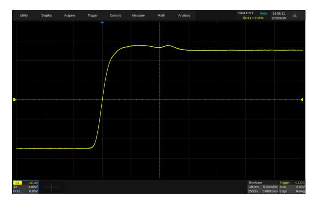
Trig Pos, timebase is changed to 5 ns/div, the grid number of delay (-2div) remains fixed, while the horizontal delay changes to -10 ns
