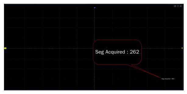
In Sequence mode, there is no waveform displayed on the screen until the acquisition is completed. During acquisition, there is a counter on the screen indicating the number of segments that have been acquired.
