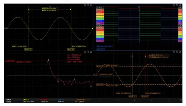
**XY** -- In XY mode, used to measure the vertical volts or amperes of source group C1-C2 (depending on the unit setting of the channel). This mode supports 4 cursors (XY\_X1、XY\_X2、XY\_Y1、XY\_Y2).
