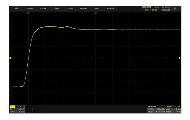
Ref Pos, timebase is changed to 5 ns/div, the horizontal delay value remains fixed, while the grid number of delay changes to -4div
