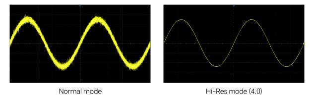
Hi-Res acquisition does not require the signal to be periodic, nor does it require stable triggering, but due to the digital filtering, the system bandwidth of the oscilloscope will degrade. The higher the enhanced bits, the lower the bandwidth. The following table shows the relationship between enhanced bits and bandwidth:
