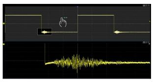
Adjust the horizontal position of the waveform by dragging the gray area of the main window left and right.
