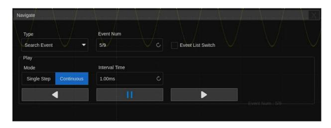
Click the *Event List Switch* area to turn the list on or off. The list contains time labels for each event. Clicking a row in the list automatically jumps to the corresponding event. This operation is equivalent to specifying an event in the *Event Num* area.
