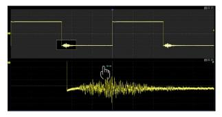
Adjust the horizontal position of the zoom area by dragging left and right in the zoom area of the main window or waveform in the Zoom window.
