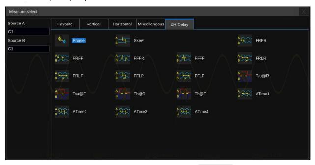
In the parameter selection area, the channel corresponding to  $Source\ A$  is specified first, and then the channel corresponding to  $Source\ B$ . Finally, the measurement parameter is selected. For example, to activate the skew between C1 and C2, you can follow the following steps:
