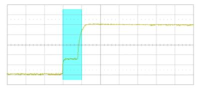
With a simple edge trigger, it is unlikely to trigger consistently on this anomaly. Thanks to the high waveform update rate of the device, we can confirm there is bus contention happening by enabling the persistence display, as shown in the figure below:
