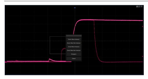
Now, we can accurately capture the exact bus contention waveform:
