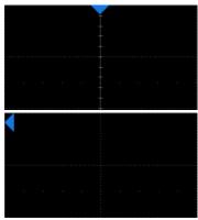
**Trigger Delay Indicator** locates where the waveform triggers on the horizontal axis. When the trigger position is outside the screen, the direction of the triangle changes to point outside the screen.
