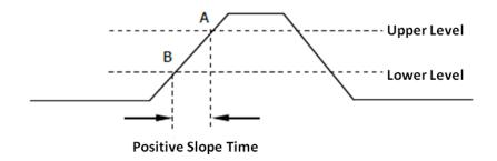
Click the Source area to select the trigger source, and click the Slope area to select rising or falling.
