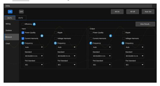
A. Efficiency Analysis for input/ output signal
