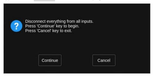
The oscilloscope will not respond to any operation until the self-cal is finished. After the self-cal is completed, click the screen to exit.
