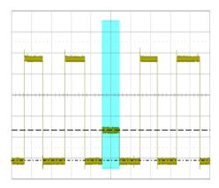
First, set the trigger type to Runt to trigger on the runt pulse. See the section "Runt Trigger" for details.
