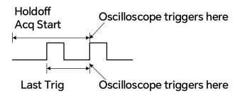
Acq Start -- The initial position of holdoff is the first-time point satisfying the trigger condition. In the example above, each holdoff starts from the first rising edge of the pulse sequence, the triggering interval is always greater than one pulse cycle.
