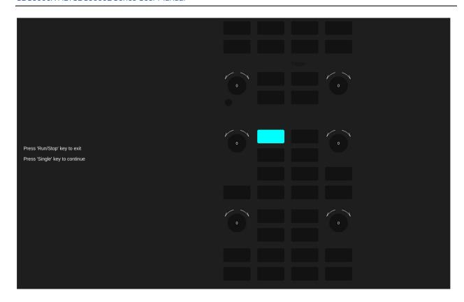
Press Single button and the first LED on the front panel will light. The corresponding position of the key on the screen will also change color. Press the Single button to check the next button.
