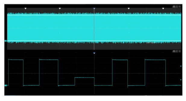
Perform Acquire > Run/Stop to stop the acquisition, and then follow the steps Analysis > Navigate > Type to select "Search Event". The following figure shows the first dwarf pulse. In this example, the list is enabled and the time labels of each event are shown in the list.
