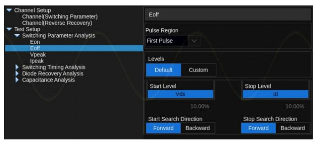
Vpeak -- Measures the peak voltage during turn-off. Configuration is the same as Eoff.
