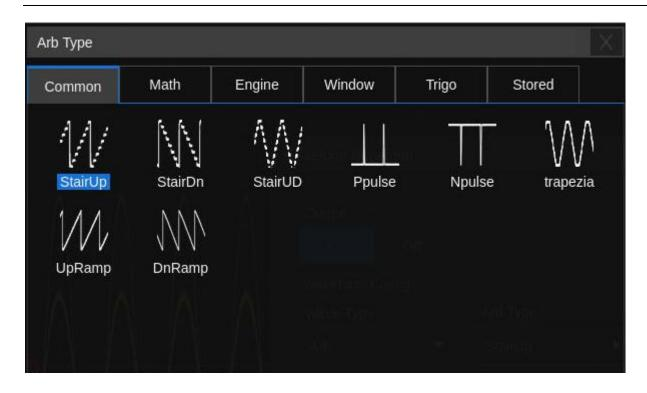
There are 6 tabs in the window. Under each tab, a catalog of waveforms is listed. Built-in waveforms are stored in Common, Math, Engine, Window, and Trigo. Stored waveforms are located in the Stored menu.
