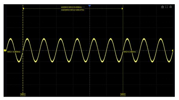
Fixed position, timebase is changed to 1ms/div, the grid number of MX1 and MX2 cursors (-4div, 2div) remains fixed. The value of MX1 and MX2 is changed to -4ms, 2ms.
