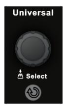
When the parameter setting area is highlighted, the Universal Knob A can be used to adjust the parameter. Press the knob to select an option from the list. The default function of the Universal Knob is to adjust the intensity of the waveform traces.
