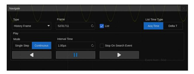
The following is an example of an occasional runt signal to demonstrate how to quickly locate and find events of interest by using the combination of Search and Navigate:
