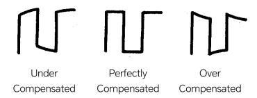
5. Use a non-metallic driver to adjust the low-frequency compensation adjustment hole on the
