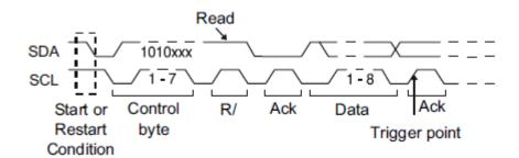
**7 Address & Data** — the oscilloscope will be triggered on the read or write frame in 7-bit address mode.
