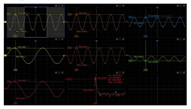
**Measure** -- Automatically indicates the measured item using cursors. and the measurement cursor cannot be adjusted. This mode supports 4 cursors (MEA1 to MEA4).
