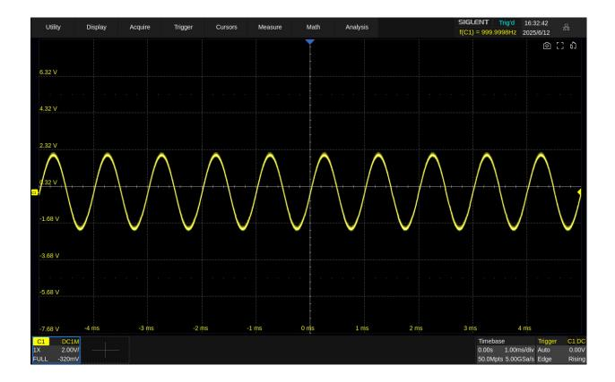
Enable axis label display, the axis label is located on the left side of the screen.
