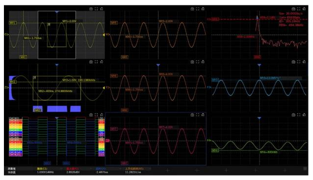
**Track** -- A set of track cursor contains two cursors. Only horizontal cursor TX is adjustable, while the vertical cursor TY automatically attach to the cross-point of the cursor and the source waveform. This mode supports 8 cursors (TX1 to TX8)
