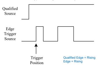
Click the *Qualify Setting* region to set the qualified source and threshold; Click the *Edge Setting* region to set the edge trigger source, threshold, and slope.
