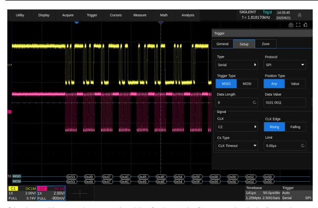
If the data width is set to be greater than 8 bits (such as 16 bits), measure the clock idle time between 8-bit data packets as 12 us, and then set the timeout time to a value between 12 and 150 us. In this example, it is set to 15 us:
