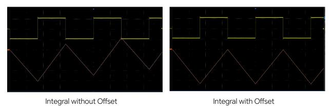
In addition, the integral operation can be performed within a specified gate. Click | Analysis | > Analysis Gate | to enable the gate function, then set | Gate A | and | Gate B | to define the gate. See "Analysis Gate" for details.
