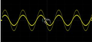
Pinch and spread the waveform vertically to rescale the vertical gain
