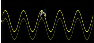
Drag the waveform up and down to move it on the vertical axis
