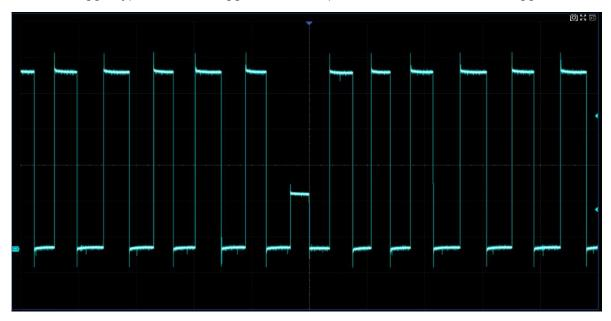
Then turn on the Search function and operate Copy from Trigger in the search dialog box so that the oscilloscope searches for the dwarf pulses according to the same setting as the trigger.
