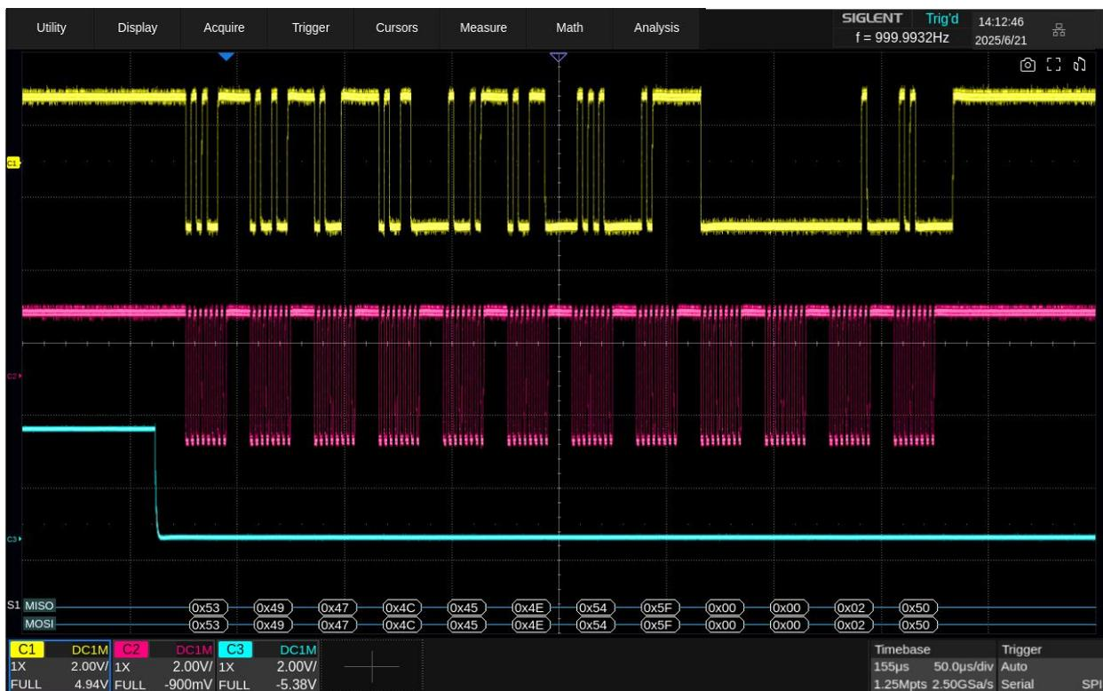
When the CS type is set to Clock Timeout, turn on Cursor, measure the clock idle time between frames as 150 µs, and measure the interval between clock pulses as 1.28 µs, then set the timeout to a value between 1.28 µs and 150 µs. In this example it is set to 5 µs:
