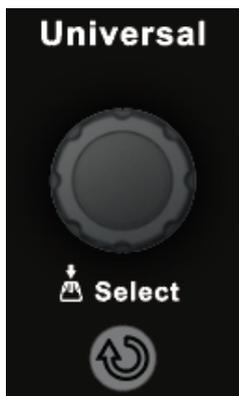
When the parameter setting area is highlighted, the Universal Knob A can be used to adjust the parameter. Press the knob to select an option from the list. The default function of the Universal Knob is to adjust the intensity of the waveform traces.
