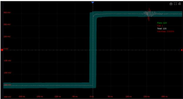
The oscilloscope utilizes a hardware-based Mask Test function, performing up to 28,000 Pass / Fail decisions each second. It is easy to generate user-defined test templates to provide trace mask comparisons, making it suitable for long-term signal monitoring or automated production line testing
