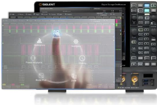
12.1" capacitive touch screen on the SDS5000X HD, supporting multi-touch gestures, can move or scale the waveform traces quickly by finger-touch movements, which greatly improves the operational efficiency
