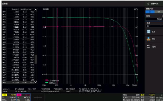
The oscilloscope can control the SIGLENT isolated USB AWG module or a stand-alone SIGLENT SDG generator, to scan the amplitude and phase-frequency response of the DUT, and display the data as a Bode Plot. This makes it possible to replace expensive network analyzers in some applications
