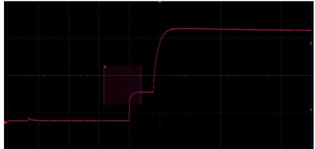
Zone Trigger is available for advanced triggering. Combine spatial triggering with common trigger modes to isolate signals of interest
