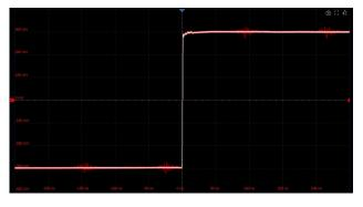
Segmented memory collection will store the waveform into multiple memory segments (up to 170,000) and each segment will store a triggered waveform as well the dead time information. The interval between segments can be as small as 1.5  $\mu$ s. All of the segments can be played back using the History function
