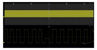
The oscilloscope can search events specified by the user in a frame based on hardware. Events flagged by the Search can be recalled automatically using Navigate. It can also navigate by time (delay position) and history frames
