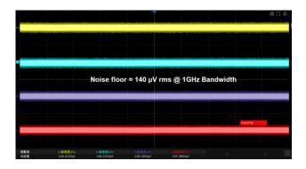
Low noise floor: 140  $\mu V rms$  at 1 GHz bandwidth
