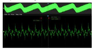
Using hardware-based Zoom technique and record length of up to 2.5 Gpts, users can select a slower timebase without compromising the sample rate, and then quickly zoom in to focus on the area of interest
