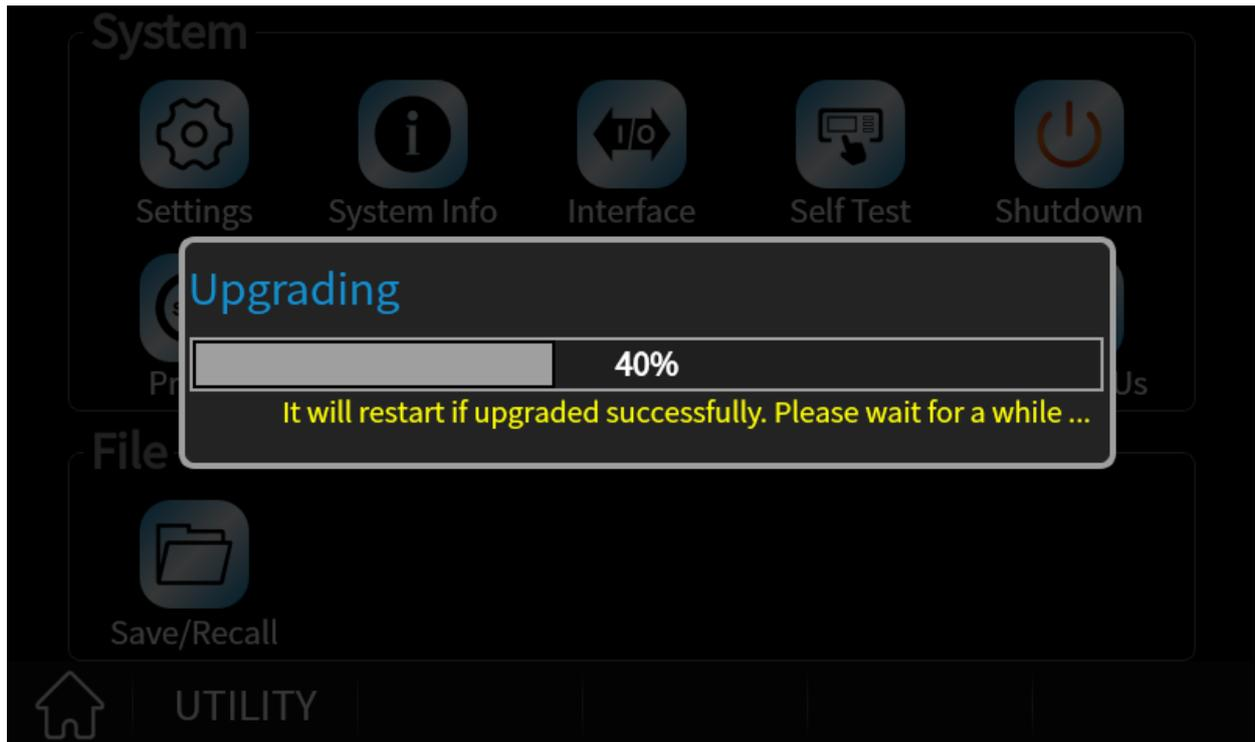
5. After the instrument reboots, check the version number through the **Utility** -> **System Info** to confirm if the upgrade is successful.
