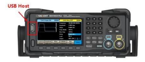
2. Press the Utility key on the front panel, and then softkey "System -> Page 1/2 -> Firmware Update", to enter the interface of the file browser.
