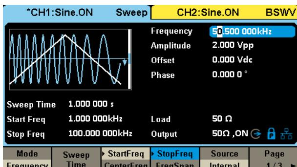
Supports two sweep modes, frequency and amplitude, to easily implement frequency sweep and amplitude sweep tests.
