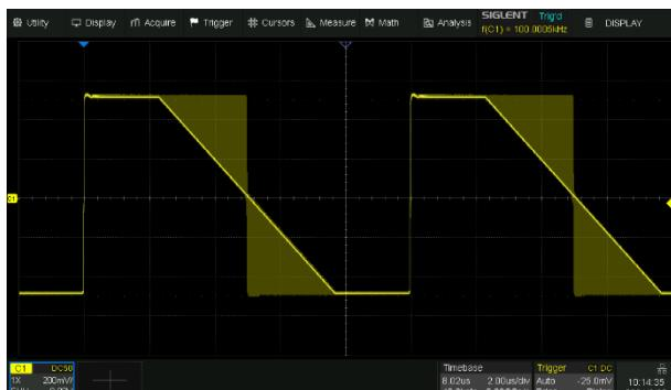
The rise/fall times can be set independently to the minimum of 10ns at any frequency and to the maximum of 22.4s. The adjustment step is as small as 100 ps.
