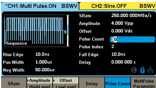
Supports up to 30 pulses, each pulse can be independently set with pulse edge and positive and negative pulse width.
