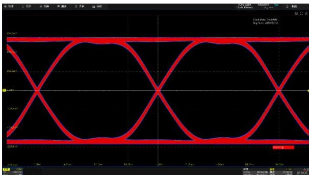
Provides PRBS3 ~ PRBS32 multiple pattern outputs, the rate is arbitrarily adjustable between  $10^{-6}$  bps ~ 40 Mbps, and the edge is arbitrarily adjustable between 10 ns ~ 1us.
