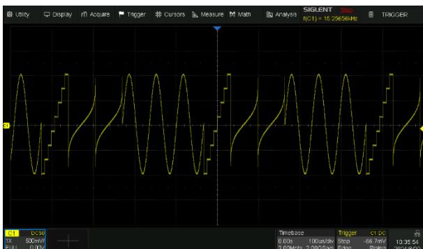
Provides sequence playback function to easily meet various testing needs. Maximum waveform storage depth reaches 8 Mpts/ch.
