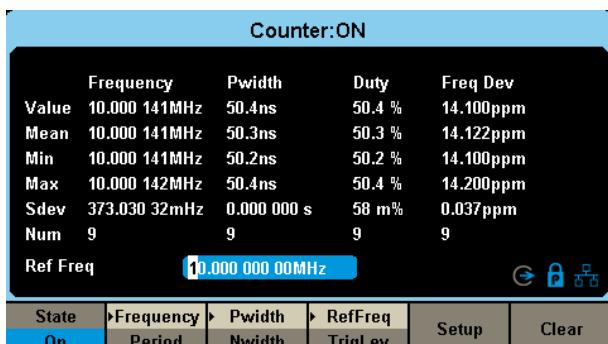
High-precision frequency counter, capable of testing the frequency range of 0.1Hz~200MHz.
