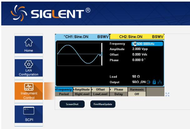
Supports instrument control through a web browser, allowing testing tasks to be completed remotely.
