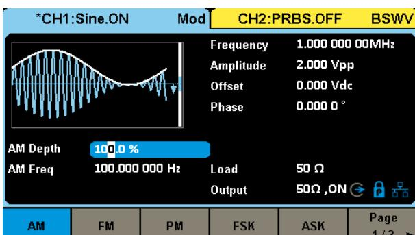
Rich modulation functions, supporting commonly used AM/DSB-AM/ FM/ PM/ ASK/ FSK/ PSK/ PWM modulation methods.
