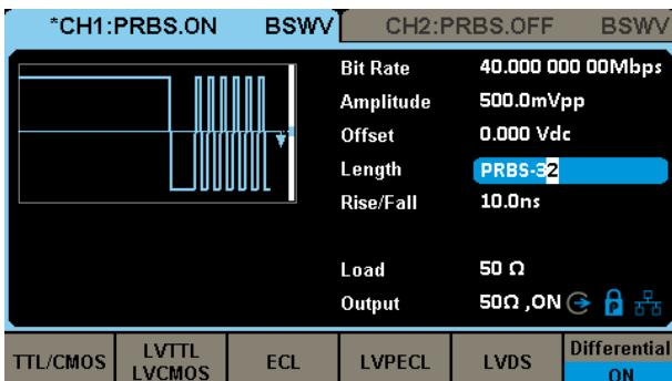
Quickly select preset level logic such as TTL, LVCMS, LVPECL and LVDS. Differential mode allows you to easily set up two channels as a differential pair output.
