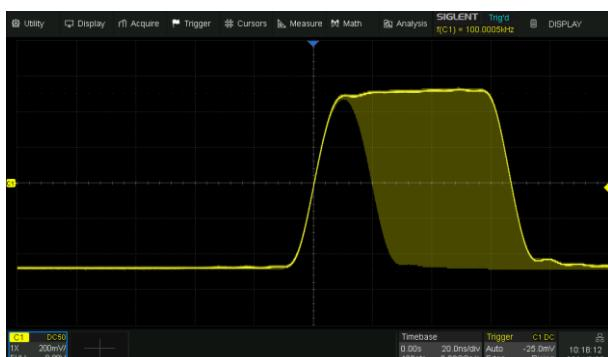
The Pulse width can be fine-tuned to the minimum of 19.4ns with the adjustment step as small as 100ps
