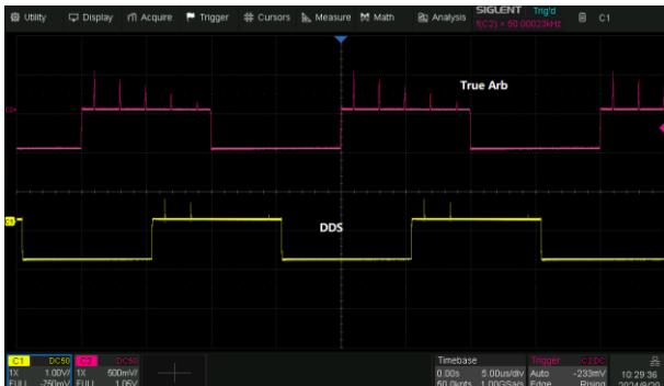
For arbitrary waveforms, TrueArb not only has all the advantages of traditional DDS, but also eliminates the probability that DDS may cause serious jitter and distortion. TrueArb generates arbitrary waveforms point by point, never skips any point so that it can reconstruct all the details of the waveform as defined.
