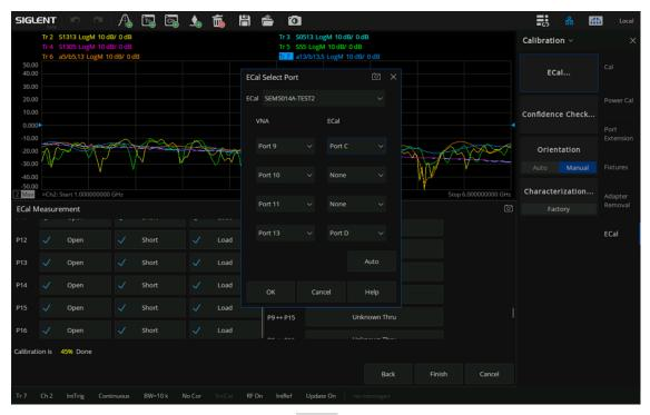
8) After completing the P9-P13 calibration, Finish will be highlighted on the UI. And then you can click Finish to end the full 16 ports calibration, as shown in the following figure.
