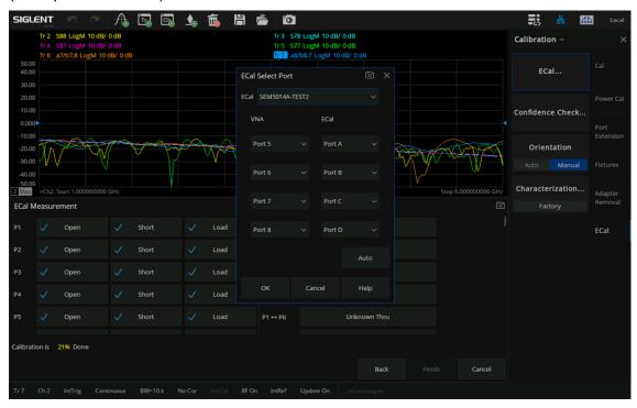
5) **P9-P12 Calibration**: Connect Ports 9, 10, 11 and 12 of matrix switch to Ports A, B, C and D of SEM5014 through SMA cables. Click OK and then click any calibration standard option of P9 (like Open/Short/Load) to start P9-P12 calibration as shown below.
