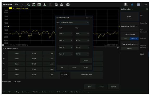
4) **P5-P8 Calibration**: Connect Ports 5, 6, 7 and 8 of matrix switch to Ports A, B, C and D of SEM5014 through SMA cables. Click OK and then click any calibration standard option of P5 (like Open/Short/Load) to start P5-P8 calibration as shown below.
