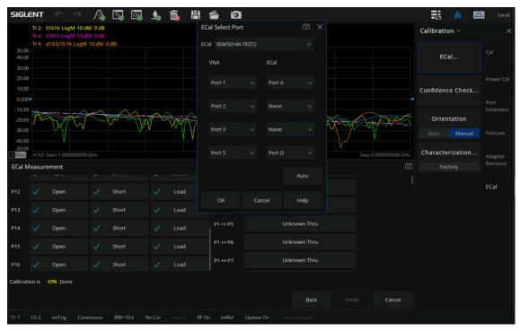
P1-P9 Calibration: Connect Ports 1 and 9 of matrix switch to Ports A and D of SEM5014 through SMA cables. Click the P1-P9 Unknown thru tab on UI and set Port 1 corresponding to Port A of Ecal, Port 2 corresponding to None of Ecal, Port 3 corresponding to None of Ecal, and Port 9 corresponding to Port D of Ecal. Click OK to perform through calibration of P1-P9, as shown below.
