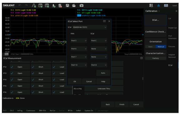
P9-P13 Calibration: Connect Ports 9 and 13 of matrix switch to Ports C and D of SEM5014 through SMA cables. Click the P9-P13 Unknown thru tab on UI and set Port 9 corresponding to Port C of Ecal, Port 10 corresponding to None of Ecal, Port 11 corresponding to None of Ecal, and Port 13 corresponding to Port D of Ecal. Click OK to perform through calibration of P9-P13, as shown below.
