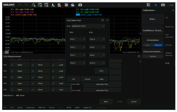
P1-P13 Calibration: Connect Ports 1 and 13 of matrix switch to Ports A and D of SEM5014 through SMA cables. Click the P1-P13 Unknown thru tab on UI and set Port 1 corresponding to Port A of Ecal, Port 2 corresponding to None of Ecal, Port 3 corresponding to None of Ecal, and Port 13 corresponding to Port D of Ecal. Click OK to perform through calibration of P1-P13, as shown below.
