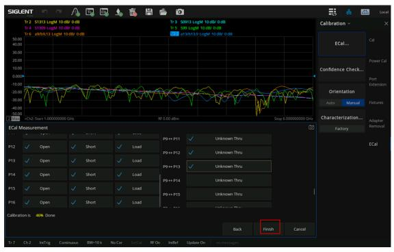
9) After calibration, you can add several traces and set S-parameter, such as S22, S88, S1616, to check the calibration effect, as shown in the following figure.
