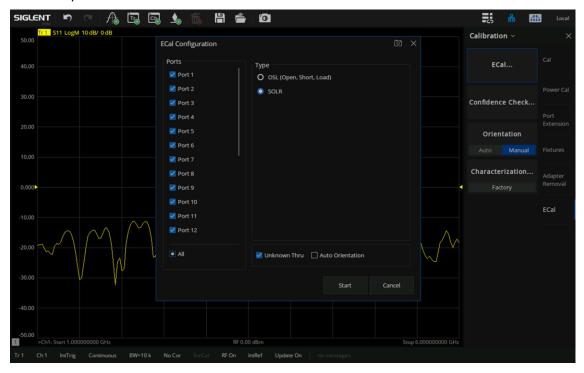
P1-P4 Calibration: Connect Ports 1, 2, 3 and 4 of matrix switch to Ports A, B, C and D of SEM5014 through SMA cables. Click OK and then click any calibration standard option of P1 (like Open/Short/Load) to start P1-P4 calibration as shown below.
