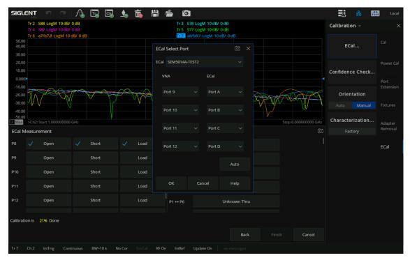
6) **P13-P16 Calibration**: Connect Ports 13, 14, 15 and 16 of matrix switch to Ports A, B, C and D of SEM5014 through SMA cables. Click OK and then click any calibration standard option of P13 (like Open/Short/Load) to start P13-P16 calibration as shown below.
