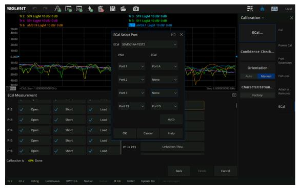
P5-P13 Calibration: Connect Ports 5 and 13 of matrix switch to Ports C and D of SEM5014 through SMA cables. Click the P5-P13 Unknown thru tab on UI and set Port 5 corresponding to Port C of Ecal, Port 6 corresponding to None of Ecal, Port 7 corresponding to None of Ecal, and Port 13 corresponding to Port D of Ecal. Click OK to perform through calibration of P5-P13, as shown below.
