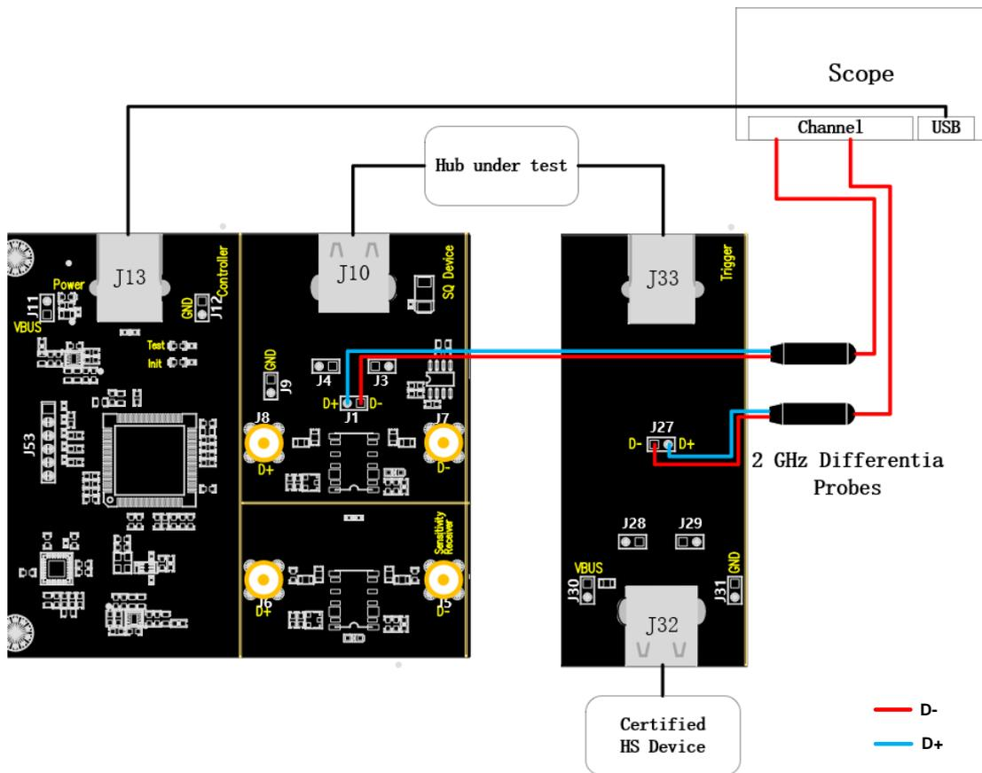
A. When using differential probes, J1 corresponds to the repeater upstream test point and J27
