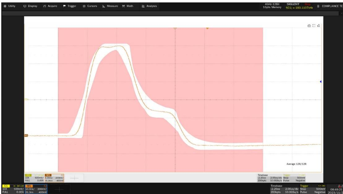
Figure 8-4 Waveform details in templates tests of points A, B, C, D
