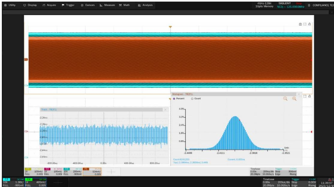
Figure 10-6 Waveform details for JTXOUT when DUT in master mode
