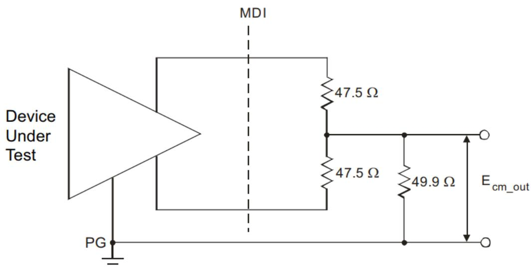
Figure 13-1 Test circuit for Common-mode output voltage
