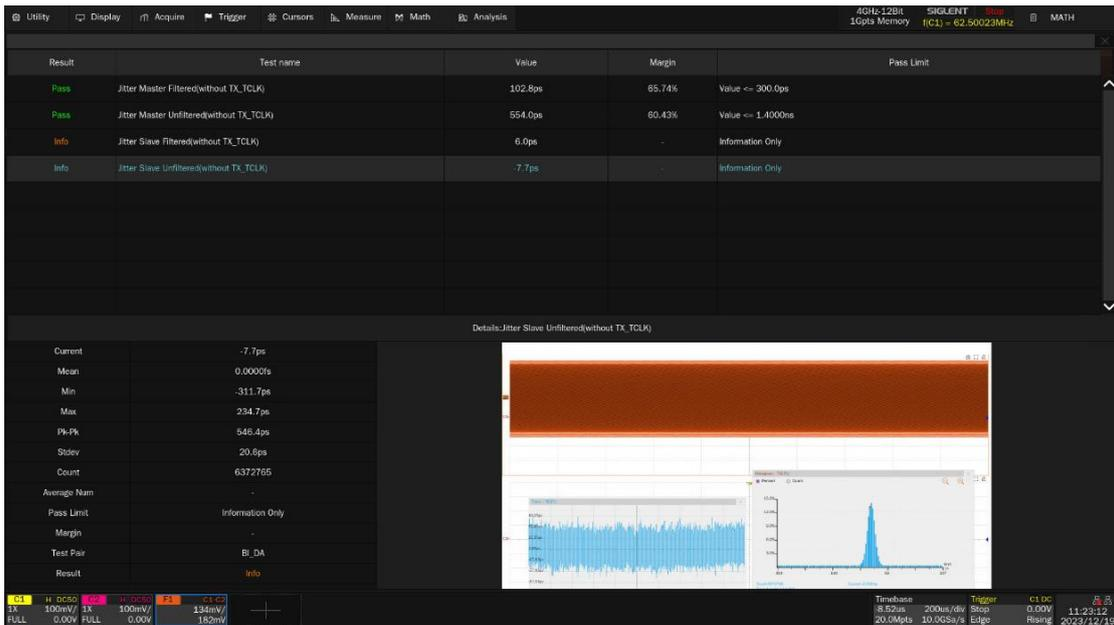
Figure 11-5 Reference results of Jitter Slave Mode Unfiltered Without TX\_TCLK
