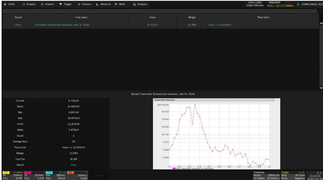
Figure 9-5 Test results of transmitter distortion tests
