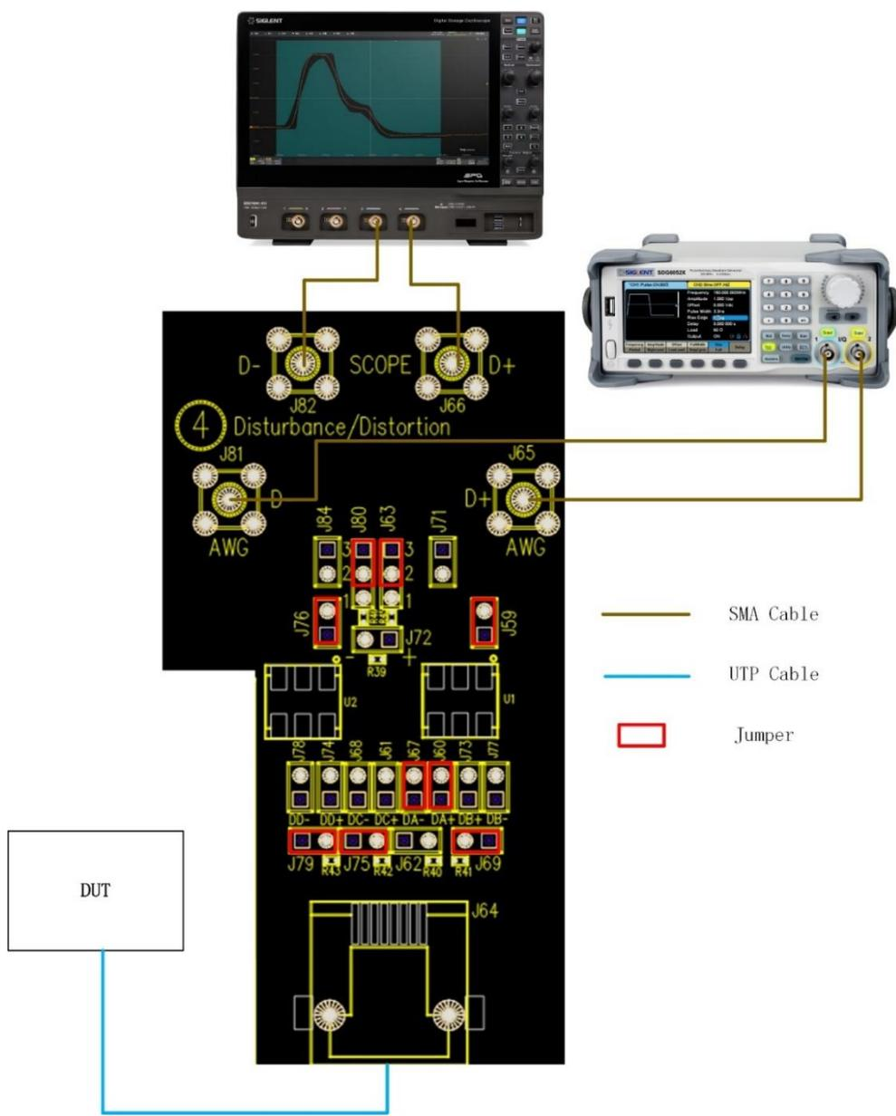
Figure 5-9 Test mode 1 and 4 test environment with disturber
