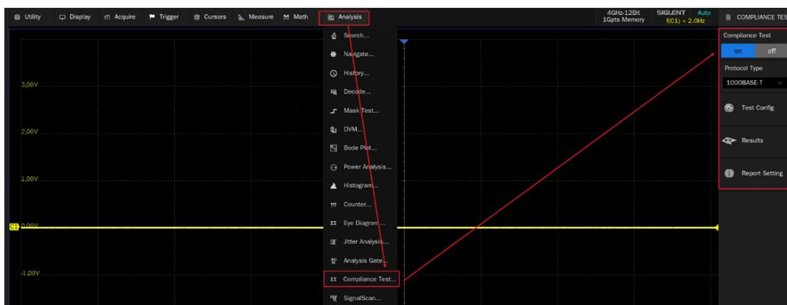
Figure 4-1 Launching 1000 BASE-T Compliance Analysis Software
