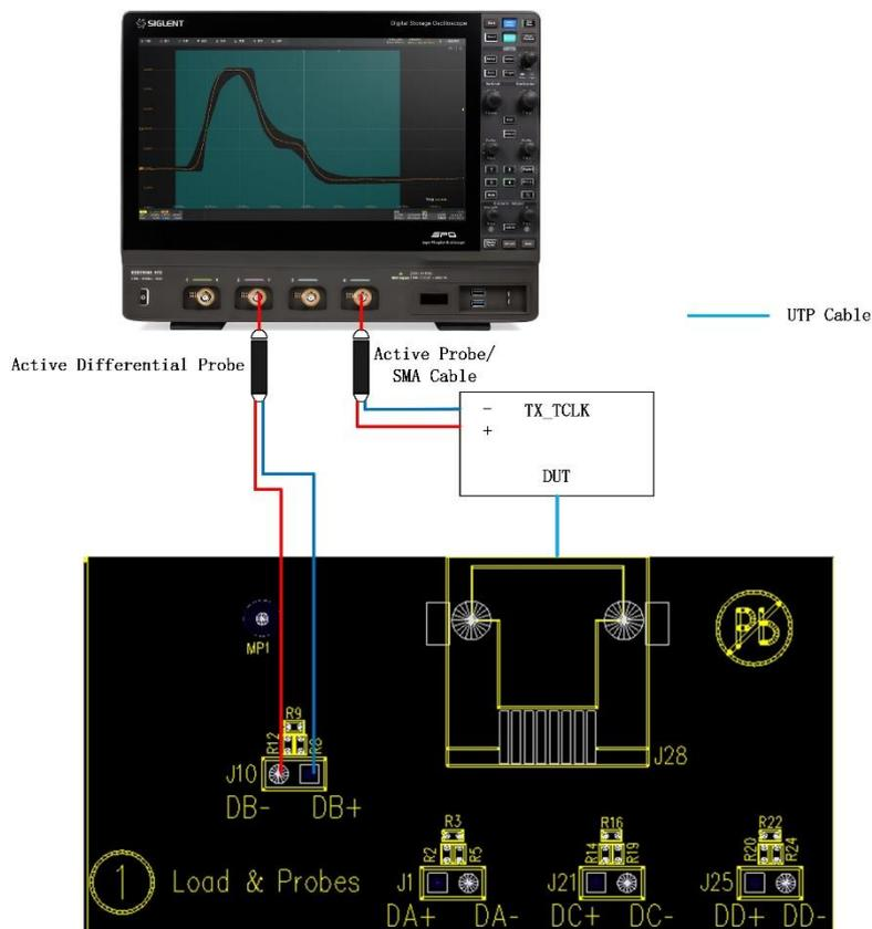
Figure 4-5 Connection diagram in the Connect menu
