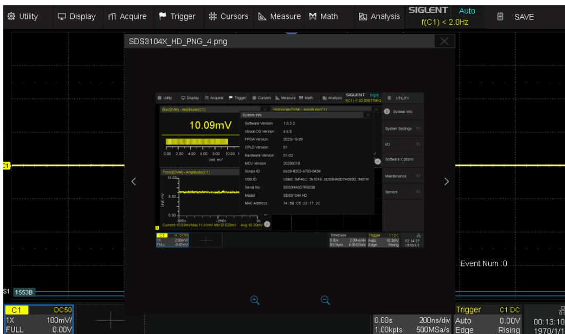
**Recall the setup file "track.xml" stored in path "Udisk0\sds3khd"**
