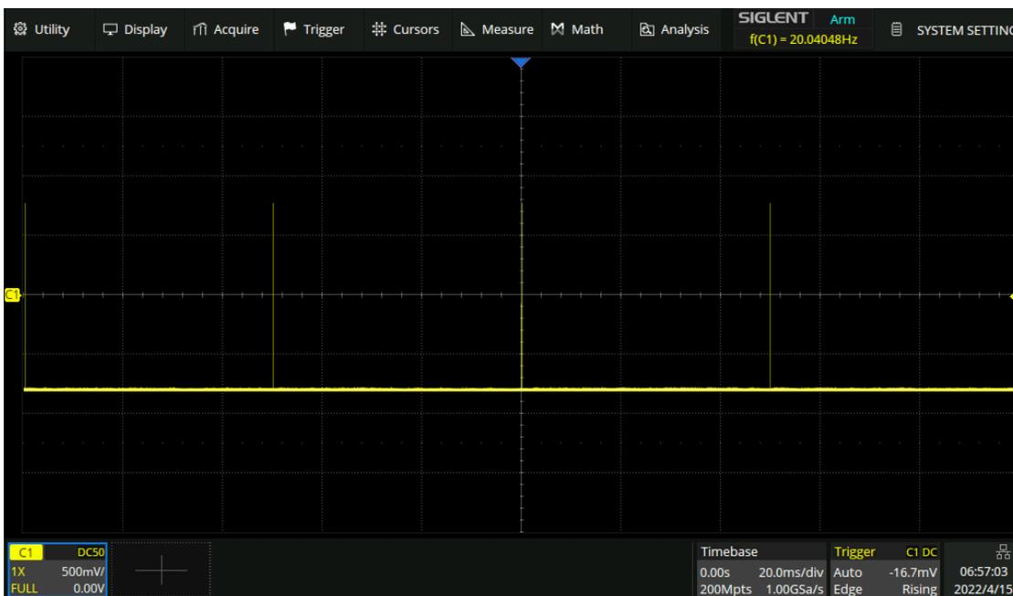
In normal mode, 5 pulses can be obtained on the screen with the sample rate of 1GSa/s at the maximum memory depth.
