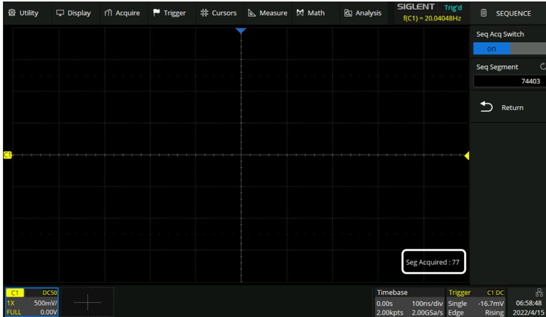
In Sequence mode, there is no waveform displayed on the screen until the acquisition is completed. During acquisition, there is a counter on the screen indicating the number of segments that have been acquired.
