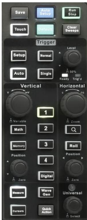
The front panel is designed to operate the basic functions without having to open the software menu. Most of the front panel controls duplicate functionality available through the touch screen but the operation is more quickly achieved.
