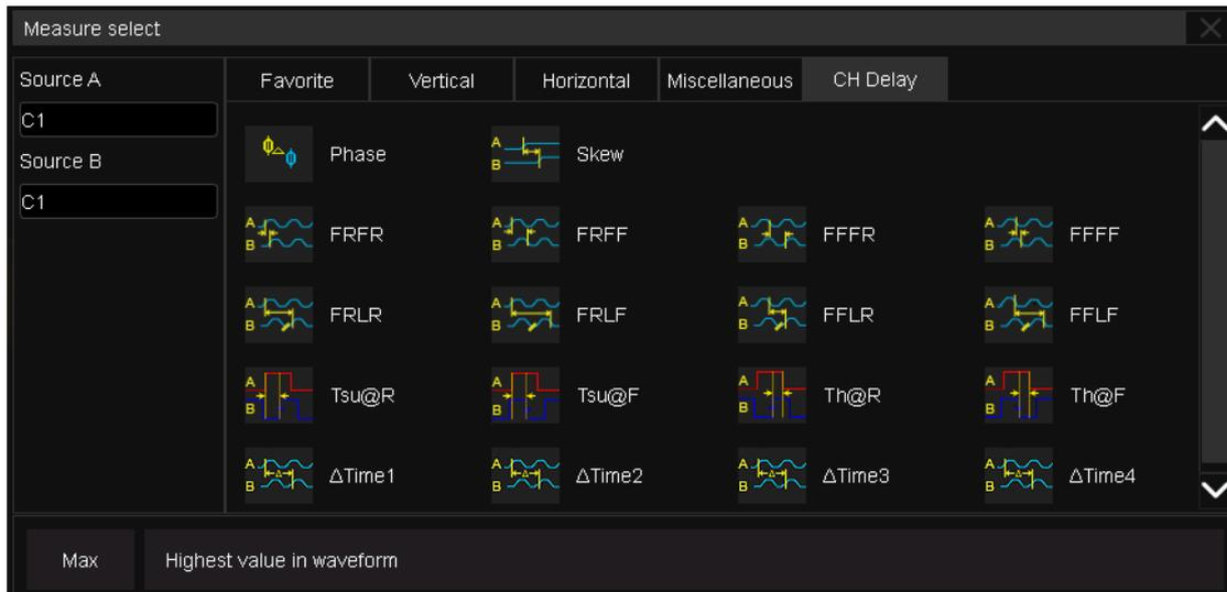
In the parameter selection area, the channel corresponding to **Source A** is specified first, and then the channel corresponding to **Source B**. Finally, the measurement parameter is selected. For example, to activate the skew between C1 and C2, you can follow the following steps:
