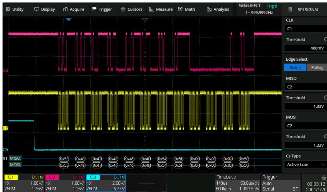
When the CS type is set to Clock Timeout, turn on Cursor, measure the clock idle time between frames as 150 us, and measure the interval between clock pulses as 1.28 us, then set the timeout to a value between 1.28 us and 150 us. In this example it is set to 5 us:
