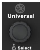
When the parameter setting area is highlighted, the Universal Knob can be used to adjust the parameter. Press the knob to select an option from the list. The default function of the Universal Knob is to adjust the intensity of the waveform traces.
