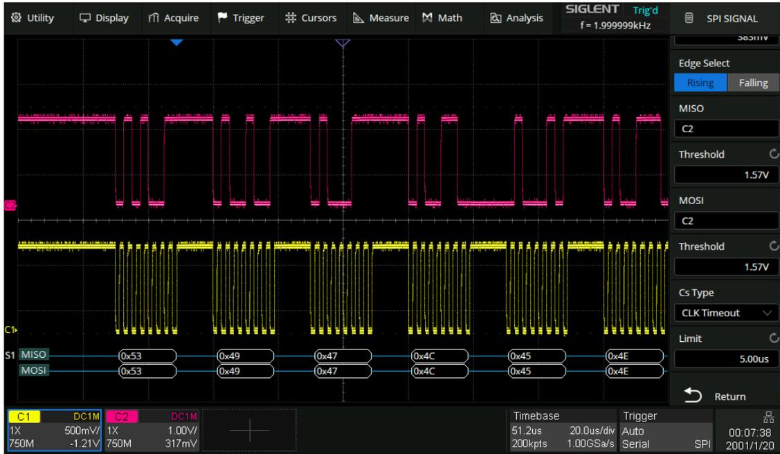
If the data width is set to be greater than 8 bits (such as 16 bits), measure the clock idle time between 8-bit data packets as 11.28 us, and then set the timeout time to a value between 11.28 and 150 us. In this example, it is set to 20 us:
