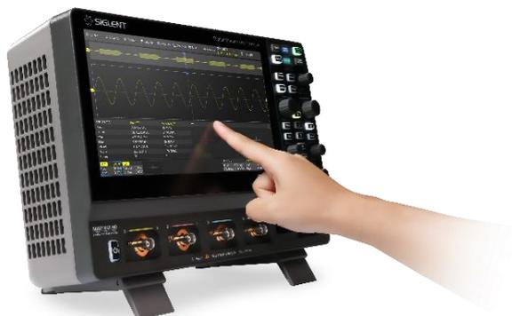
Waveforms, cursors, and trigger levels can be adjusted and a rectangular zone can be drawn by touch gestures in the grid area.
