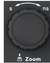
When the Zoom function is on, the waveform area is divided into upper and lower parts. The area of about 1/3 height above is the main window, and the area of about 2/3 height below is the zoom window. Touch a window to activate it. The currently activated window is highlighted by the dashed line.
