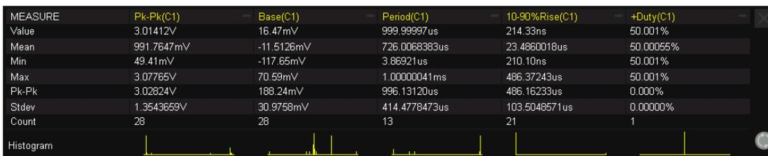
Touch the histogram area of a parameter to enlarge it for details. You can move the large histogram window position around the display by dragging. Touch the histogram of another parameter to switch to the corresponding enlarged histogram.
