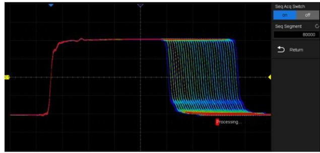
Segmented memory collection will store the waveform into multiple memory segments (up to 80,000) and each segment will store a triggered waveform as well the dead time information. The interval between segments can be as small as 2  $\mu$ s. All of the segments can be played back using the History function.
