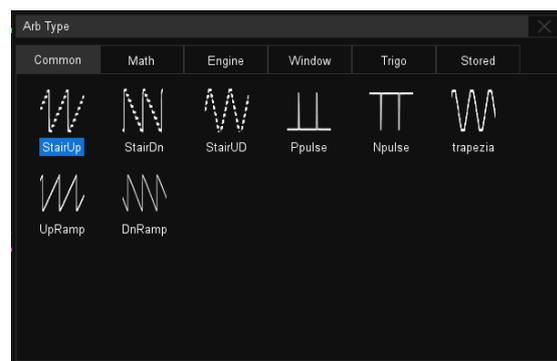
The USB waveform generator can output waveforms with up to 25 MHz frequency and  $\pm 3$  V amplitude. Six basic waveforms together with multiple types of predefined waveforms and as user-defined arbitrary waveforms are supported.
