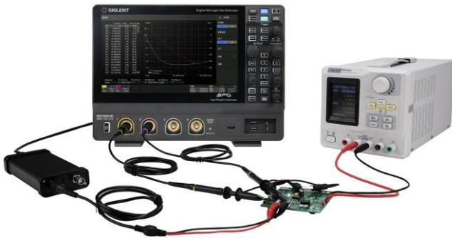
SDS1000X HD can control the USB AWG module or control an independent SIGLENT SDG instrument, scan a device's amplitude and phase frequency response, and display the data as a Bode Plot. There is also a Vari-level Mode for accurately measuring Power Supply Control Loop Response (PSRR).
