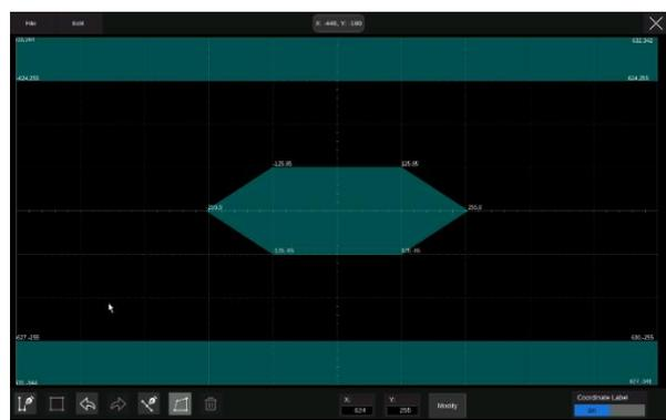
The oscilloscope utilizes a hardware-based Mask Test function, performing up to 80,000 Pass / Fail decisions each second. It is easy to generate user-defined test templates to provide trace mask comparisons, making it suitable for long-term signal monitoring or automated production line testing.
