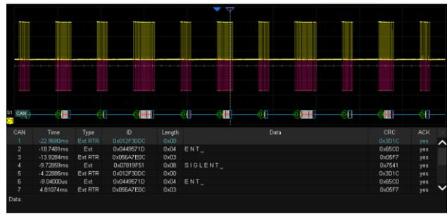
Display the decoded characters through the events list. Bus protocol information can be quickly and intuitively displayed in tabular form. I<sup>2</sup>C, SPI, UART, CAN, LIN, CAN FD, FlexRay are supported.
