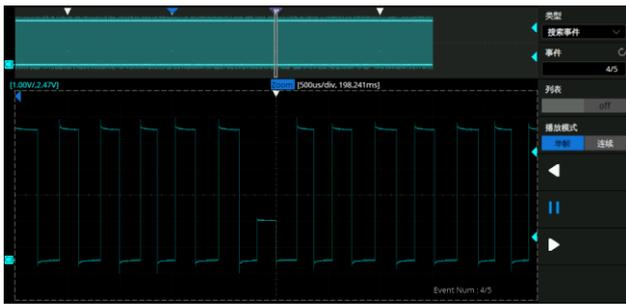
The oscilloscope can search events specified by the user in a frame. Events flagged by the Search can be recalled automatically using Navigate. It can also navigate by time (delay position) and history frames.
