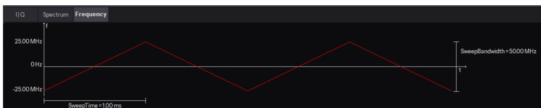
Information such as sweep time, sweep frequency and sweep bandwidth are clearly displayed in the frequency plot.
