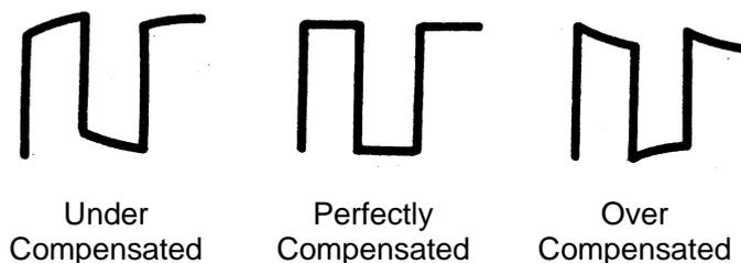
5. Use a non-metallic driver to adjust the low-frequency compensation adjustment hole on the probe until the waveform displayed is as the “Perfectly compensated” in the figure above.
