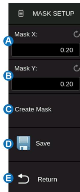
Under mask testing, the user detects signal changes by creating specific rules for the signal to be detected (including setting the horizontal and vertical adjustment range of the signal), and then observing whether the signal is outside the rule range.
