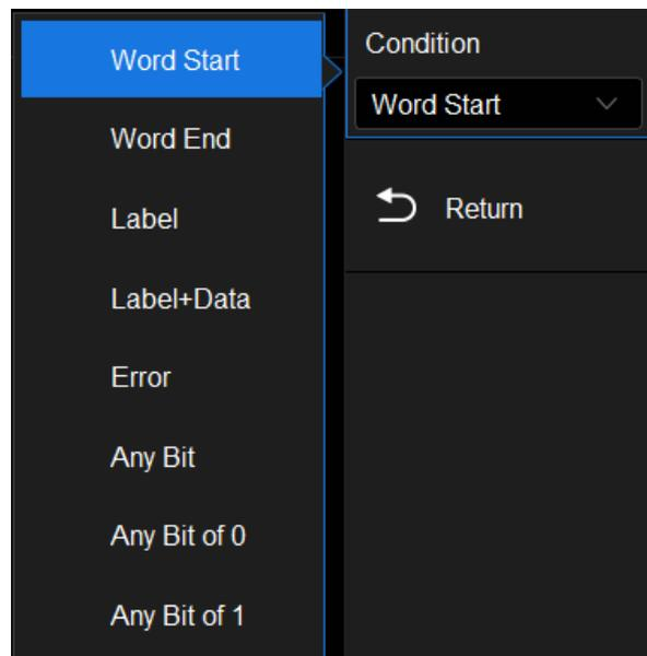
**Word Start** – The oscilloscope triggers at the start of the word.
