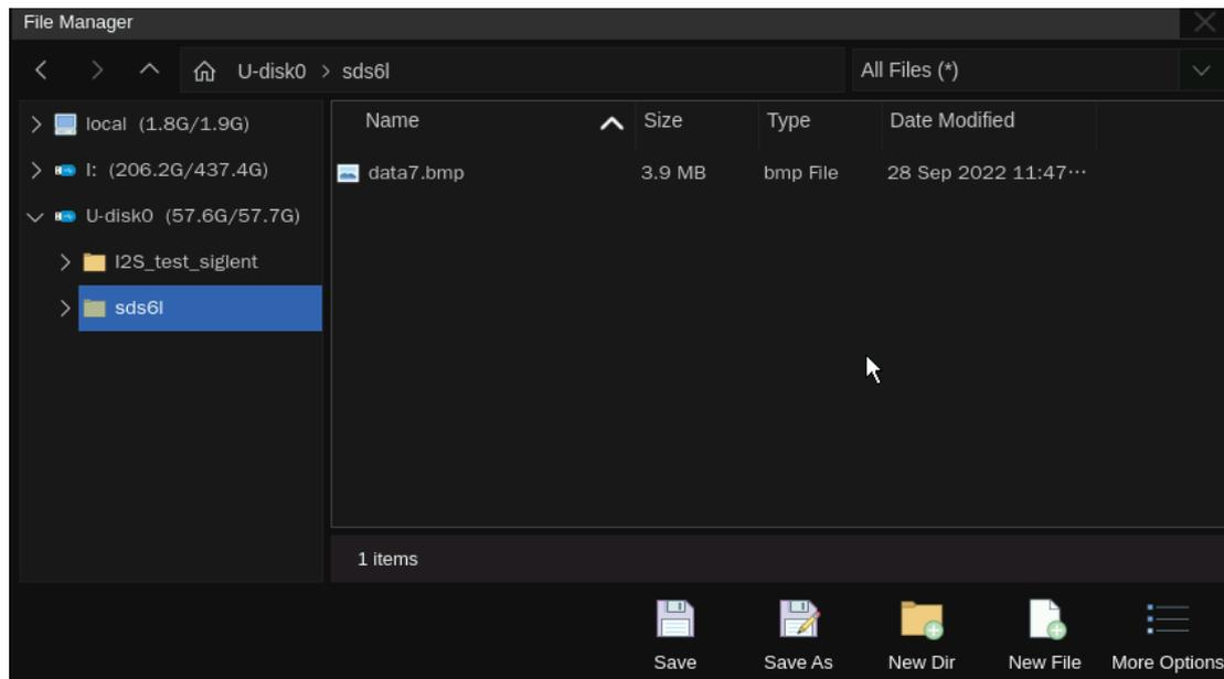
In step 4, if **Save** is selected instead of **Save As**, the system saves the file as the default file name SDS7xxxA\_BMP\_n.bmp, where n is an integer incrementing from 1. The default save path is \SIGLENT\.
