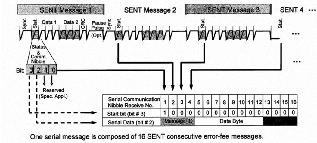
The serial message frame contains 21 bits of payload data. Two different configurations can be chosen and determined by the configuration bit (serial data bit #3, serial communication nibble No. 8):
