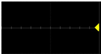
**Trigger Level Indicator** shows the level where the waveform triggers on the vertical axis.
