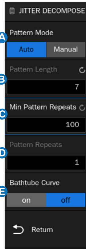
The result of jitter decomposition will be shown in the measured area. Users can add the jitter components interested, including measurement values, histogram, track, and spectrogram. Refer to the “Jitter Measure” section for details.
