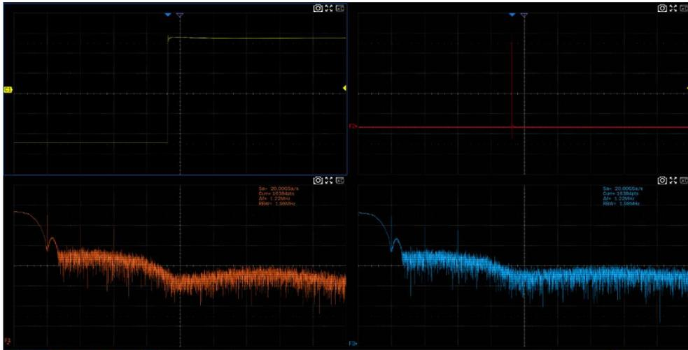
This example uses two nested operations to achieve FFT analysis of the differential operation results of C1 waveform:
