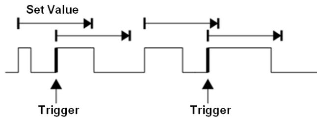
Trigger source, slope (rising, falling), limit range, and time value can be set in the trigger dialog box. Holdoff, coupling, and noise reject can be set in interval trigger, see the sections "Holdoff", "Trigger Coupling" and "Noise Reject" for details.
