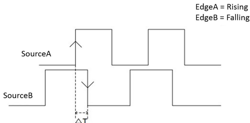
Click the **SourceB Setting** region to set the edge trigger source and slope. Click the **Limit Range** and **Upper / Lower Value** region to set the delay time condition.
