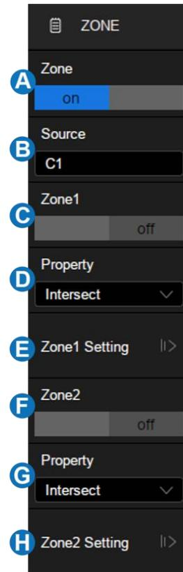
The zones can be created and moved by the mouse or by setting **Zone Setting** in the dialog box. The color of the zone’s outline is consistent with the color of the specified source (Channel 1 = Yellow, etc...).
