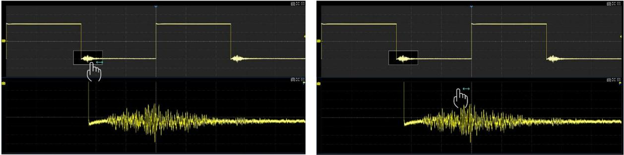
Adjust the horizontal position of the zoom area by dragging left and right in the zoom area of the main window or waveform in the Zoom window.
