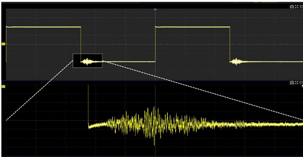
The area not covered by the gray background in the main waveform area is the range to be zoomed in (zoom area). Click the descriptor box of the zoom trace to recall the quick dialogs for setting the vertical and horizontal parameters of the zoom window.
