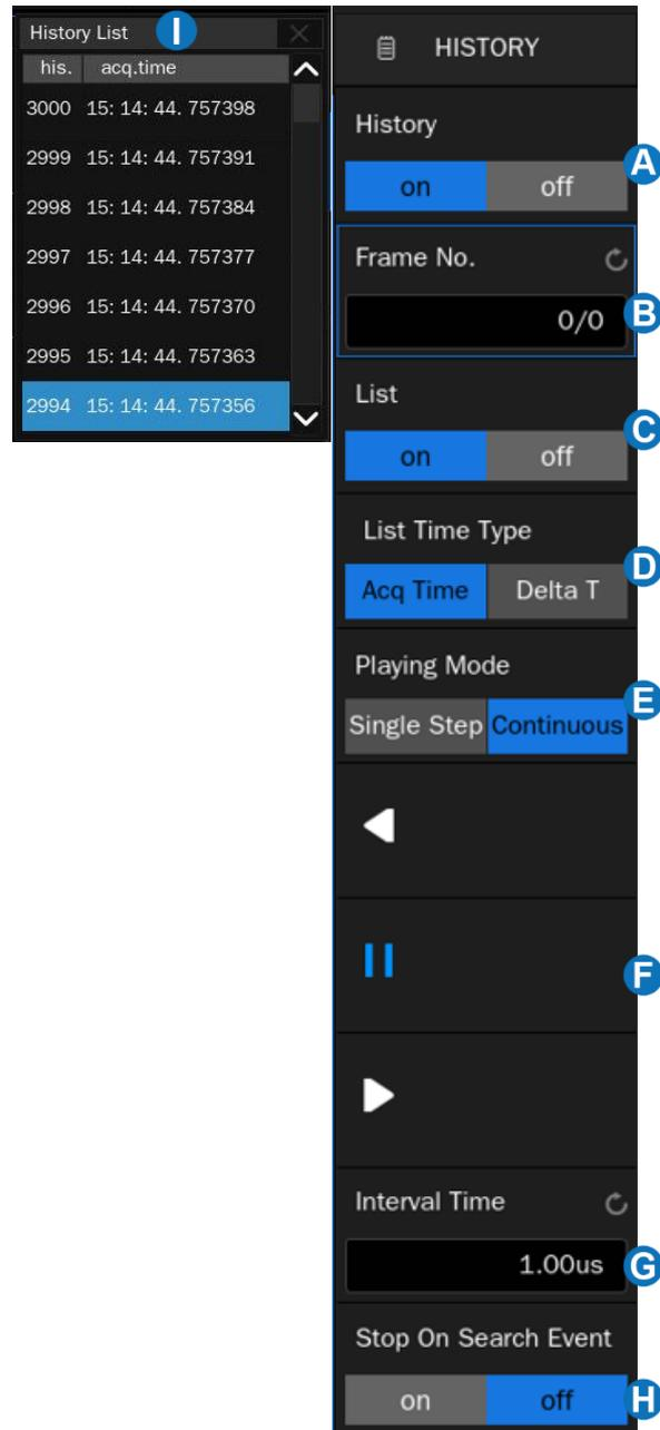
The oscilloscope automatically stores acquired frames. It can store up to 124,000 frames but the number may vary due to the memory depth and timebase settings. Turn on history mode, then the stored frames can be recalled and measured.
