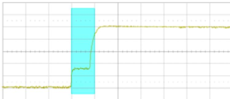
With a simple edge trigger, it is unlikely to trigger consistently on this anomaly. Thanks to the high waveform update rate of the SDS7000A, we can confirm there is bus contention happening by enabling the persistence display, as shown in the figure below:
