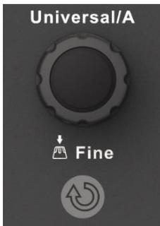
When the parameter setting area is highlighted, the Universal Knob A can be used to adjust the parameter. Press the knob to select an option from the list. The default function of the Universal Knob is to adjust the intensity of the waveform traces.
