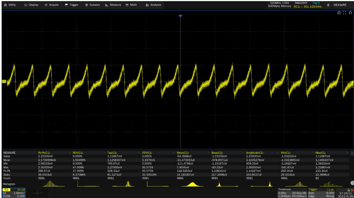
In M2 mode, up to 12 parameter measurements are displayed at a time. When statistics are enabled, they are distributed on the right side of the measurement item. Click a row to add or replace a measurement.
