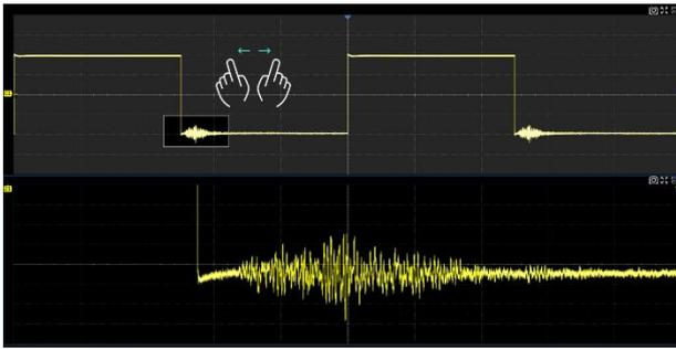
Adjust the horizontal/vertical scale of the main window by using a pinching or spreading gesture in the gray area of the main window.
