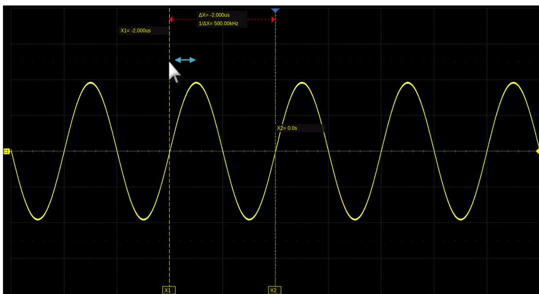
Click the display area of  $\Delta X$  (or  $\Delta Y$ ) in M1 mode and drag it to move the two cursors simultaneously, as shown in the figure below. This is equivalent to the operation on the cursor type X1-X2 or Y1-Y2.
