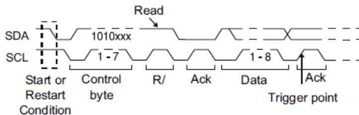
**7 Address & Data** -- the oscilloscope will be triggered on the read or write frame in 7-bit address mode.
