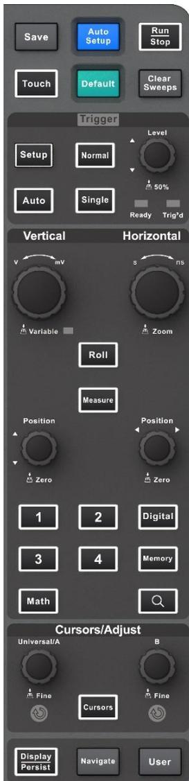
The front panel is designed to operate the basic functions without having to open the software menu. Most of the front panel controls duplicate functionality available through the touch screen display but the operation is more quickly achieved.
