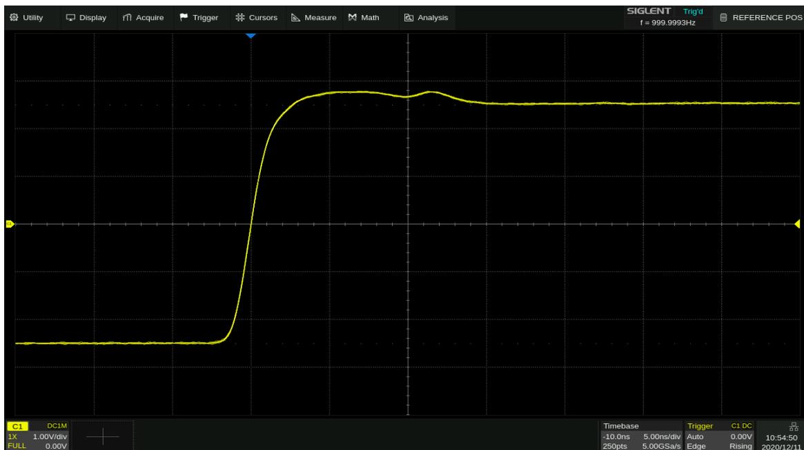
Fixed position, timebase is changed to 5 ns/div, the grid number of delay (-2div) remains fixed, while the horizontal delay changes to -10 ns
