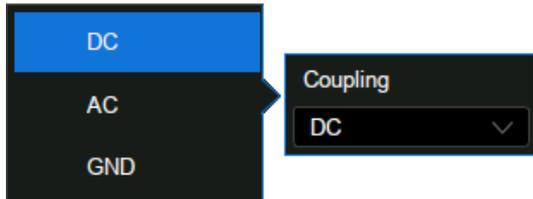
**List:** Sets parameters with more than two options, such as coupling mode of channels. Click the parameter region, and then select the expected option from the pop-up list.
