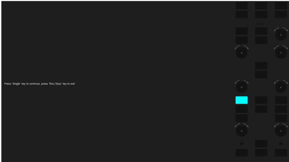
Press **Single** button and the first LED on the front panel will light. The corresponding position of the key on the screen will also change color. Press the **Single** button to check the next button.
