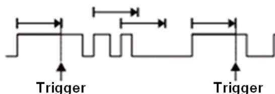
Trigger source, slope (rising, falling), dropout type, and time value can be set in the trigger dialog box. Holdoff, coupling, and noise reject can be set in the dropout trigger, see the sections "Holdoff", "Trigger Coupling" and "Noise Reject" for details.
