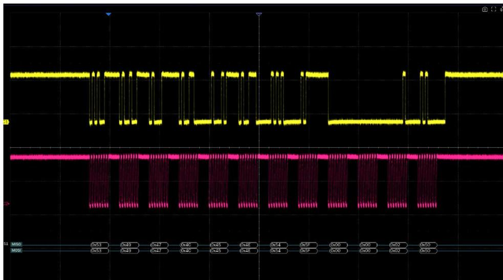
If the data width is set to be greater than 8 bits (such as 16 bits), measure the clock idle time between 8-bit data packets as 2.5 us, and then set the timeout time to a value between 2.5 and 30 us. In this example, it is set to 5 us:
