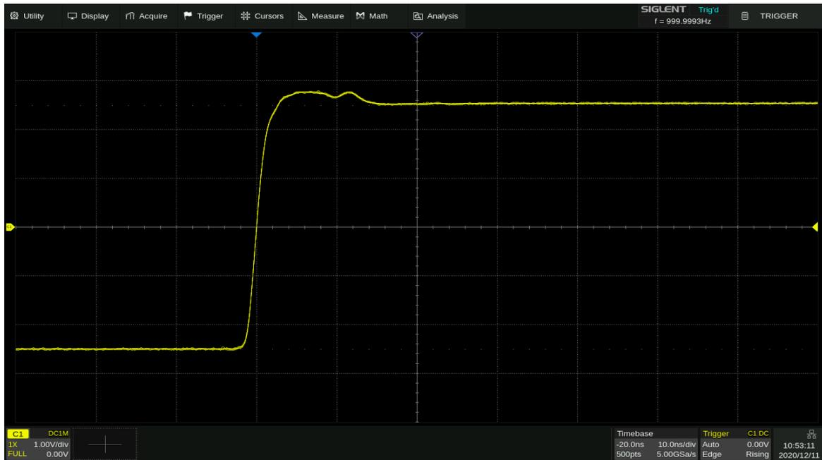
Timebase = 10 ns/div, Horizontal Delay = -20 ns = - 2 div
