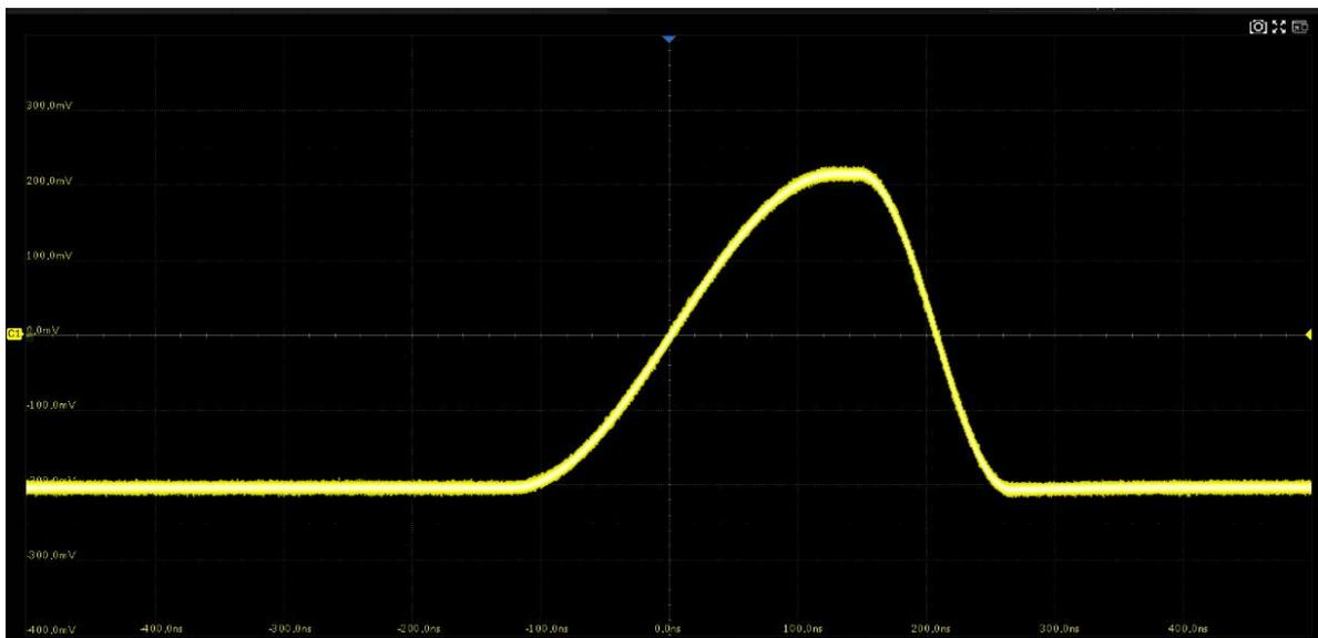
In the example, 43231 pulses can be obtained with the sample rate of 20 GSa/s at the maximum memory depth.
