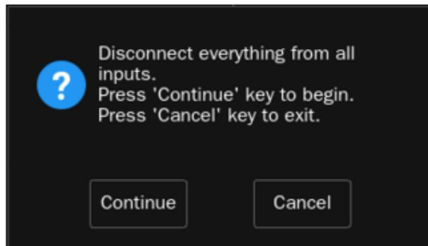
3. The oscilloscope will not respond to any operation until the self-cal is finished. After the self-cal is completed, click the screen to exit.
