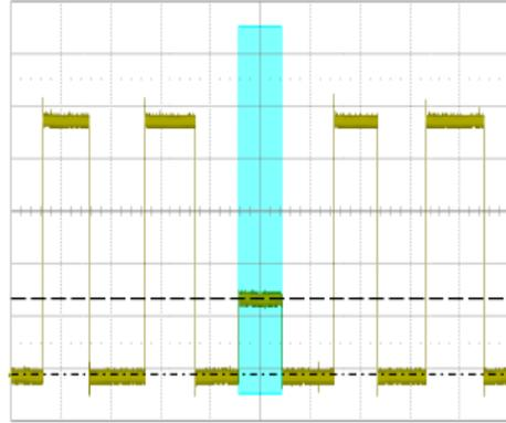
First, set the trigger type to Runt to trigger on the runt pulse. See the section “Runt Trigger” for details.
