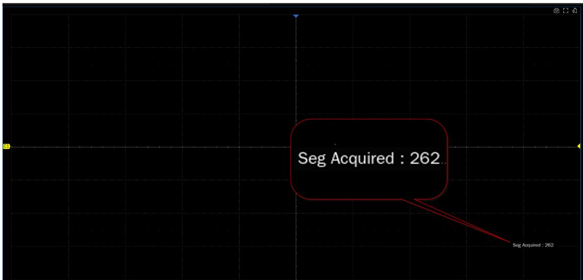
In Sequence mode, there is no waveform displayed on the screen until the acquisition is completed. During acquisition, there is a counter on the screen indicating the number of segments that have been acquired.
