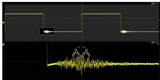
Adjust the horizontal scale of Zoom window by horizontal pinch and spread in the zoom area of the main window or the Zoom window.
