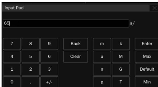
Let’s use the operation of setting the “deskew” of a channel as an example: If the expected value is 65 ns, input “65” on the virtual keypad, and then choose *n* as the unit “ns” to complete the operation. On the virtual keypad, clicking the button *Max* , *Min* , and *Default* quickly sets the parameter to the maximum, minimum, and default values.
