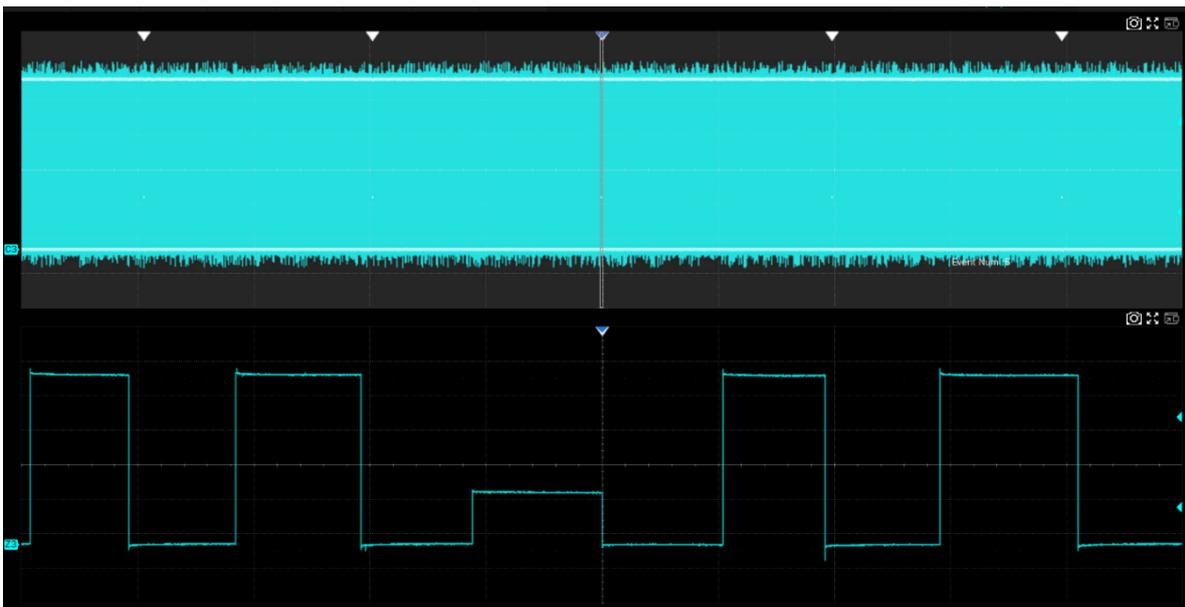
Perform **Acquire** > **Run/Stop** to stop the acquisition, and then follow the steps **Analysis** > **Navigate** > **Type** to select “Search Event”. The following figure shows the first dwarf pulse. In this example, the list is enabled and the time labels of each event are shown in the list.
