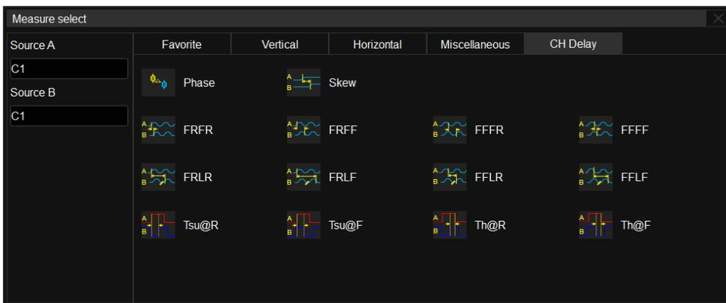
In the parameter selection area, the channel corresponding to **Source A** is specified first, and then the channel corresponding to **Source B**. Finally, the measurement parameter is selected. For example, to activate the skew between C1 and C2, you can follow the following steps:
