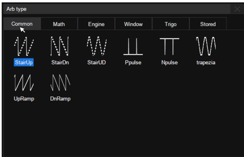
There are 6 tabs in the window. Under each tab, a catalog of waveforms is listed. Built-in waveforms are stored in Common, Math, Engine, Window, and Trigo. Stored waveforms are located in the Stored menu.
