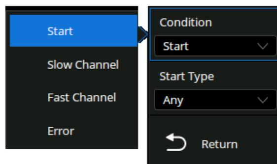
**Start** -- The oscilloscope will be triggered at the start of the message (after 56 Sync ticks). You can select the type of message: Fast Channel Message, Slow Channel Message, or any.
