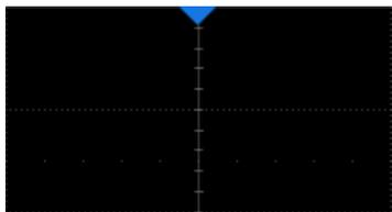
**Trigger Delay Indicator** locates where the waveform triggers on the horizontal axis. When the trigger position is outside the screen, the direction of the triangle changes to point outside the screen.
