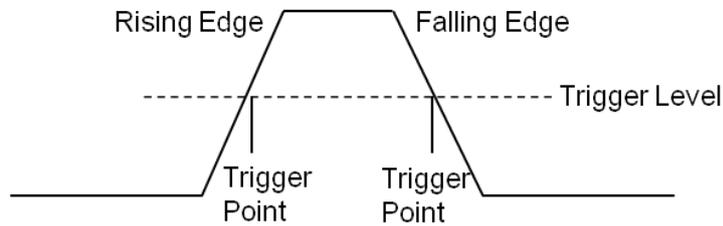
Click the **Source** area to select the trigger source, and click the **Slope** area to select rising, falling, or alternating.
