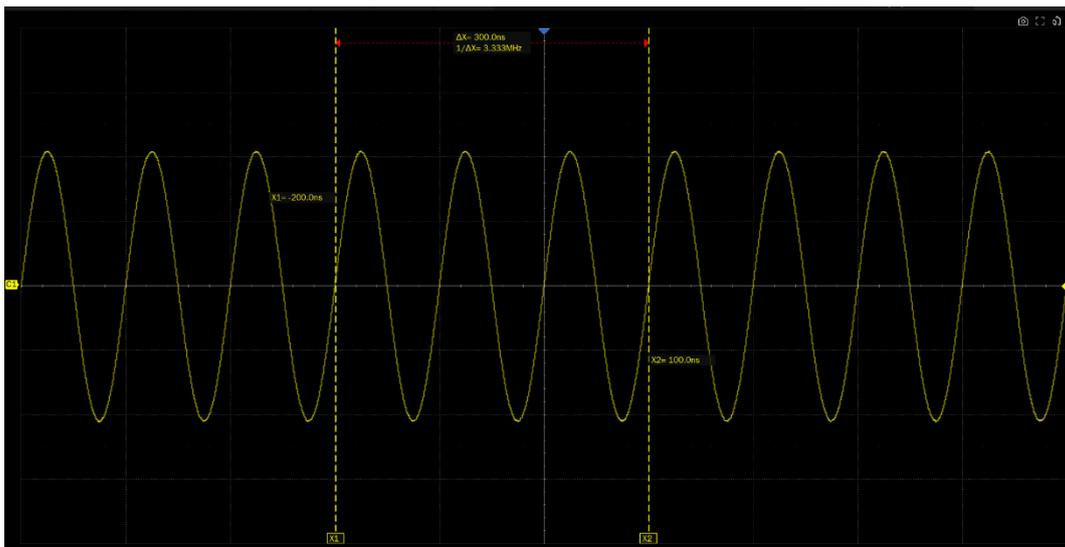
Fixed delay, timebase is changed to 100 ns/div, and the value of X cursors (-200 ns, 100 ns) remains fixed. The grid number of X cursors is changed to -2div, 1div.
