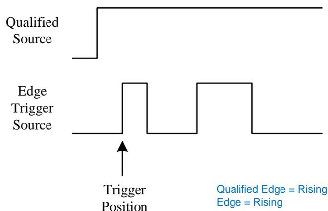
Click the **Qualify Setting** region to set the qualified source and threshold; Click the **Edge Setting** region to set the edge trigger source, threshold, and slope.
