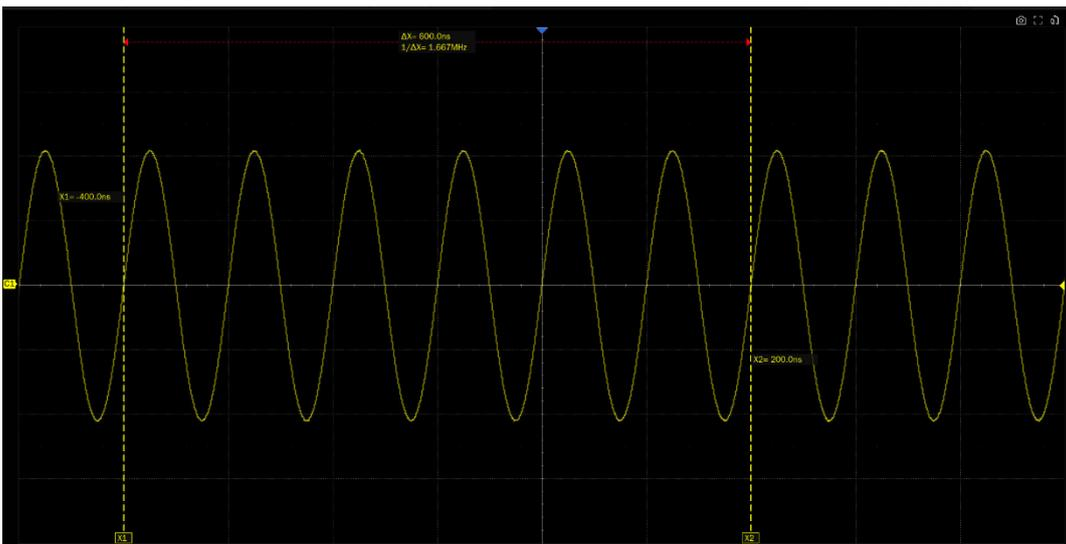
Fixed position, timebase is changed to 100 ns/div, and the grid number of X cursors (-4div, 2div) remains fixed. The value of X1 and X2 is changed to -400 ns, 200 ns.
