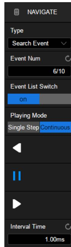
Click the **Event List Switch** area to turn the list on or off. The list contains time labels for each event. Clicking a row in the list automatically jumps to the corresponding event. This operation is equivalent to specifying an event in the **Event Num** area.
