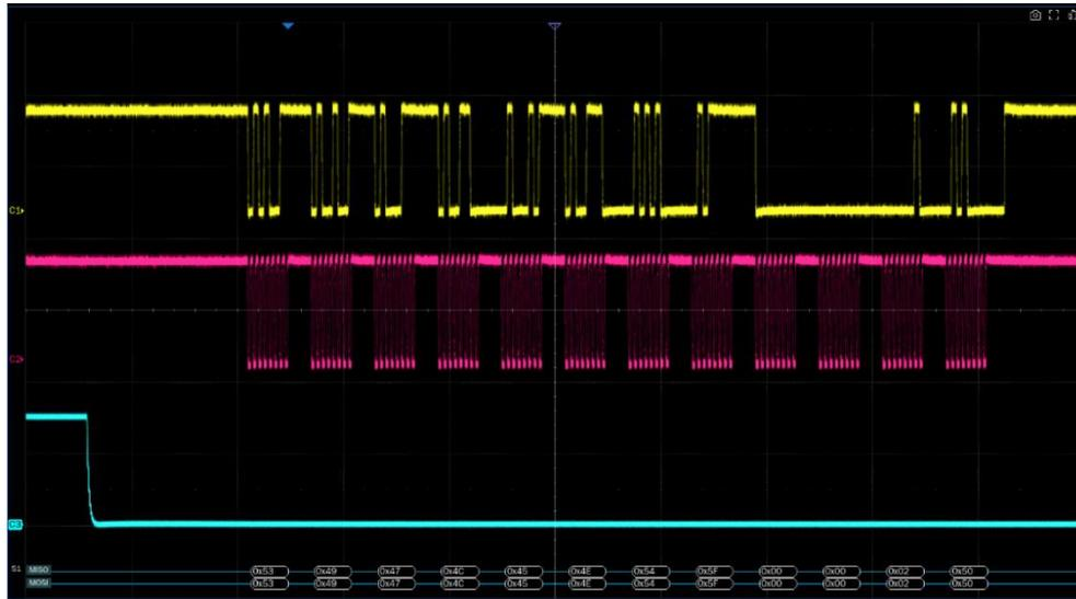
When the CS type is set to Clock Timeout, turn on Cursor, measure the clock idle time between frames as 0.3 us, and measure the interval between clock pulses as 30 us, then set the timeout to a value between 0.3 us and 30 us. In this example it is set to 1 us:
