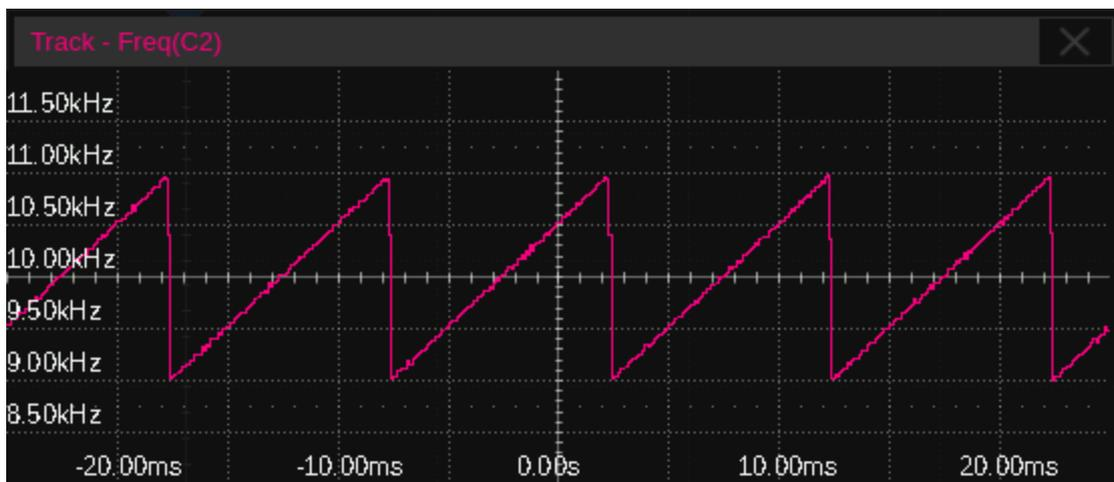
The upper limit of the statistic number in a frame is set in **Statistics** > **AIM Limit**, which means the values exceeding the limit will not be shown in the track plot. The upper limit is 1,000 by default and can be set to up to 100,000.
