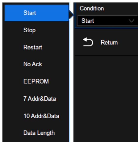
**Start** -- The oscilloscope will be triggered when the SDA line transitions from high to low while the SCL is high.
