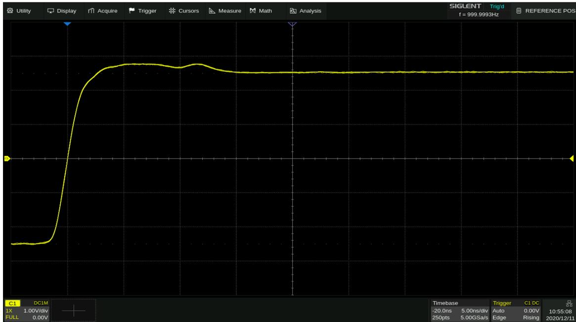
Fixed delay, timebase is changed to 5 ns/div, the horizontal delay value remains fixed, while the grid number of delay changes to -4div
