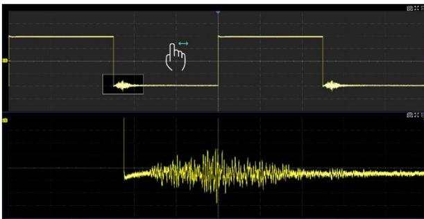
Adjust the horizontal position of the waveform by dragging the gray area of the main window left and right.
