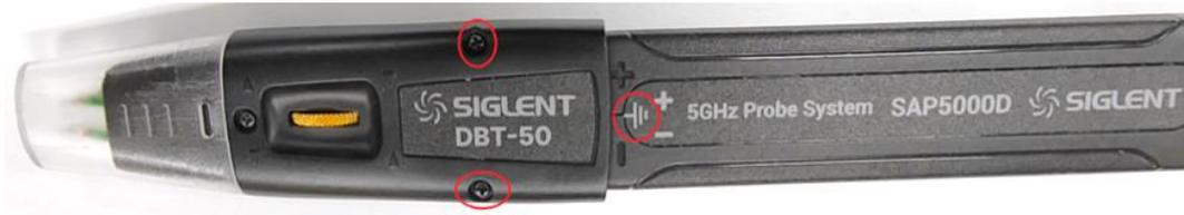
Please connect DBT-50 and probe amplifier as shown above, pay attention to the screws and grounding marks in red circles. After installation, it will look like the following picture.
